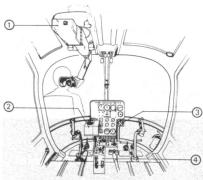
HOT installation in BO 105 hélicopter Helicopter in firing position
