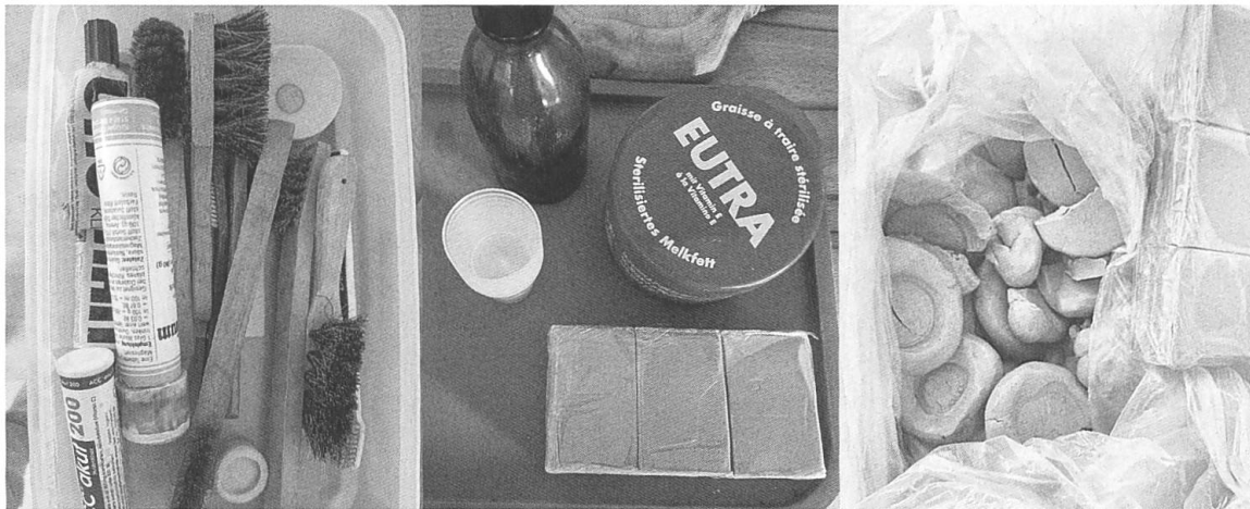
Fig. 5–7 Materials for plaster cast making- brushes and toothbrushes for smoothing, tubes from vitamin tablets for forming, «Eutra» bagbalm, adhesive, ethanol and cups for holding it, as well as plasticine (manufacturer unknown) for the moulds themselves.
