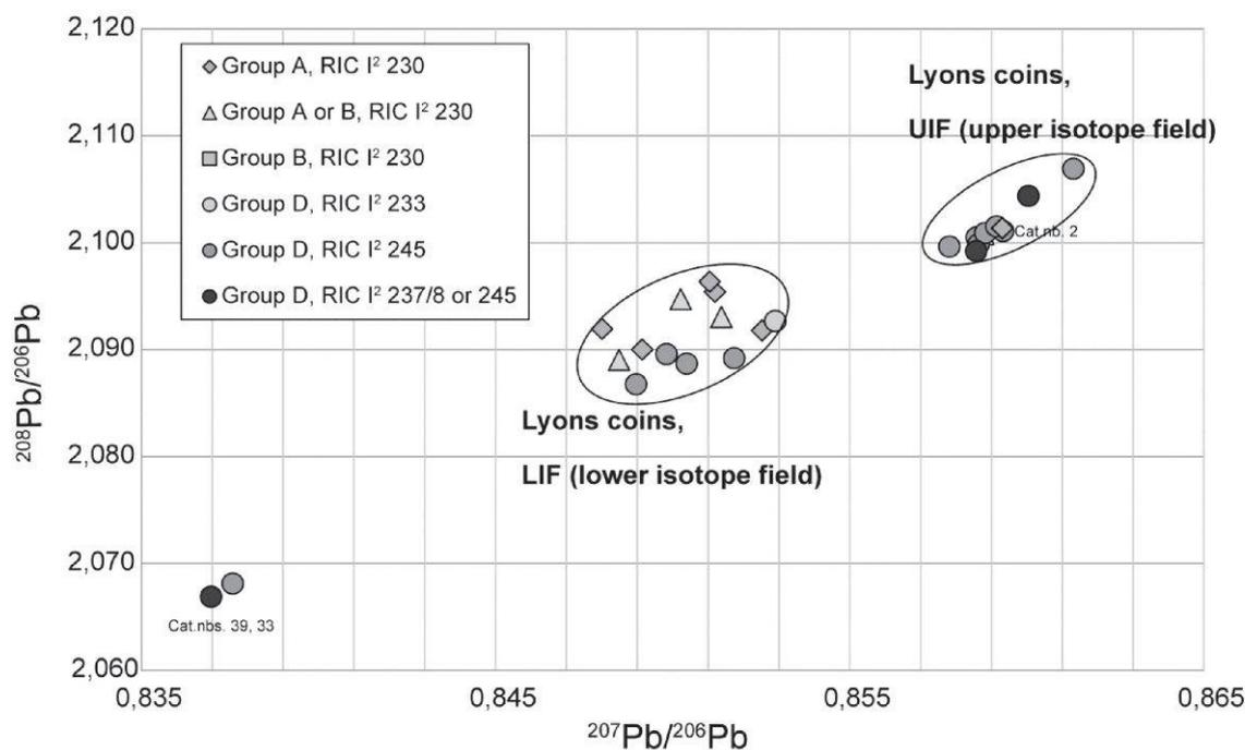
Fig. 5 Diagram  $^{207}\text{Pb}/^{206}\text{Pb}$  versus  $^{208}\text{Pb}/^{206}\text{Pb}$ , Lyon copper coins of LAS I and LAS II. The lead isotope ratios obtained by MC-ICP-MS result in two isotope fields. Isotope field UIF is dominated by LAS II coins – only one coin of LAS I (coin no. 2) plots within this field. Isotope field LIF comprises of both LAS I and LAS II coins. [Statistical errors are smaller than symbols].
