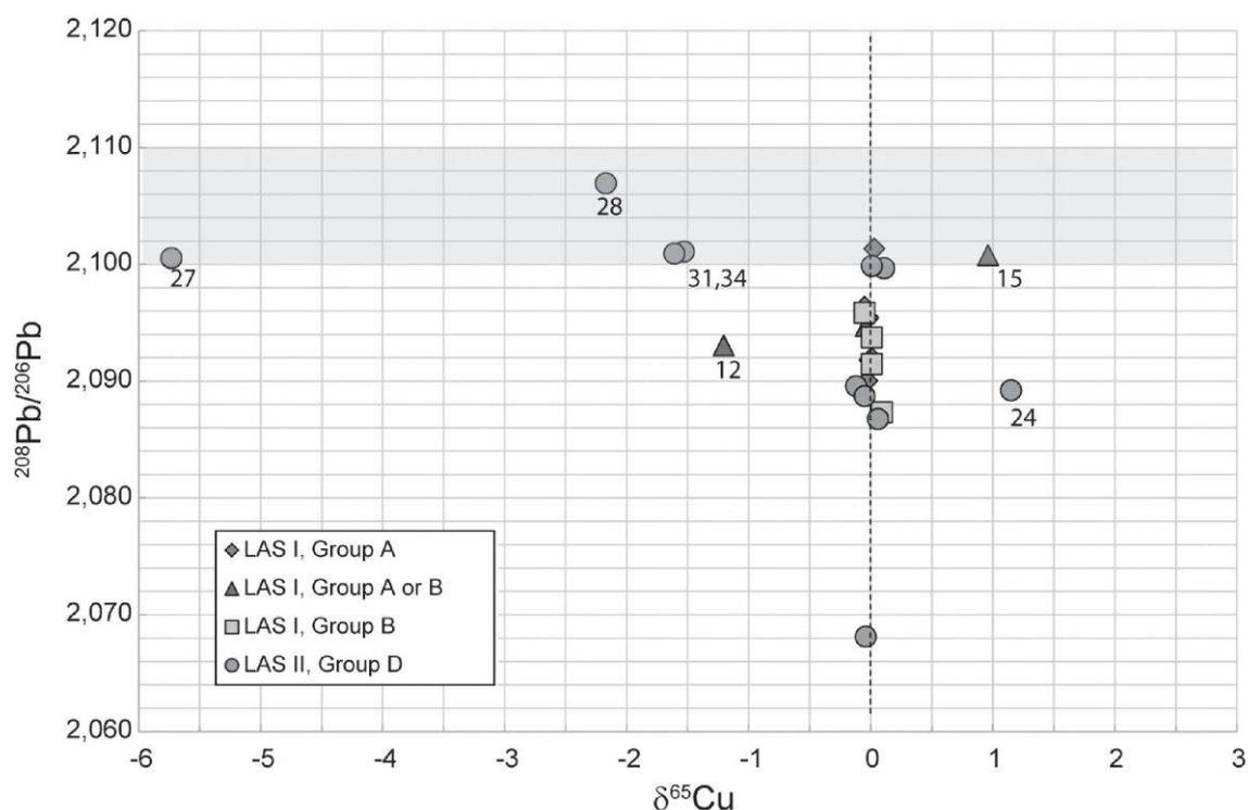
Fig. 6 Copper isotope diagram  $\delta^{65}\text{Cu}$  versus  $^{208}\text{Pb}/^{206}\text{Pb}$ . A strong accumulation of data is found along a vertical line  $\delta^{65}\text{Cu}=0\text{‰}$ . The horizontal strip (grey) represents the isotope signature of Iberian Pyrite Belt ores.
