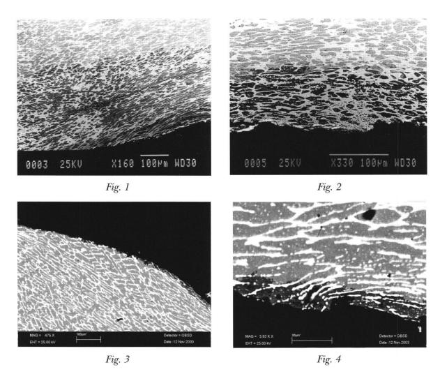
Fig. 1. Back scattered electron (BSE) image of a section through a denarius of Geta ( $\sim 50\%$  silver). The surface of the coin is towards the bottom right (see text for explanation). Fig. 2. BSE image of a section through the surface layers of the denarius of Geta. The surface is towards the bottom of the image (see text for explanation).
