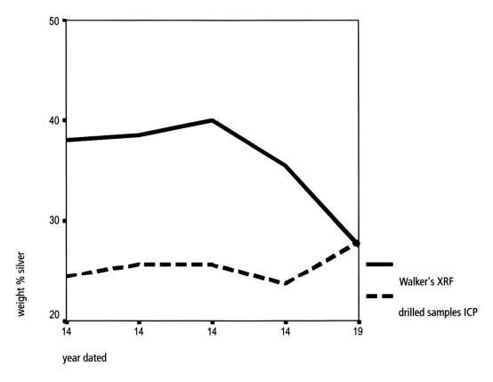
Fig. 5. Comparison of the silver contents of tetradrachms of Tiberius analysed by XRF and by ICP (same coins).
