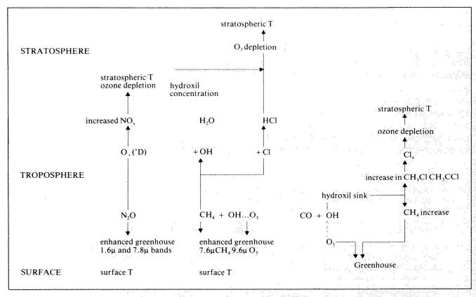
Fig. 1. Summary of the direct ettects and indirekts of Nitrous Oxide, Methane and Carbon Monoxide on the radiation balance in the atmosphere.
