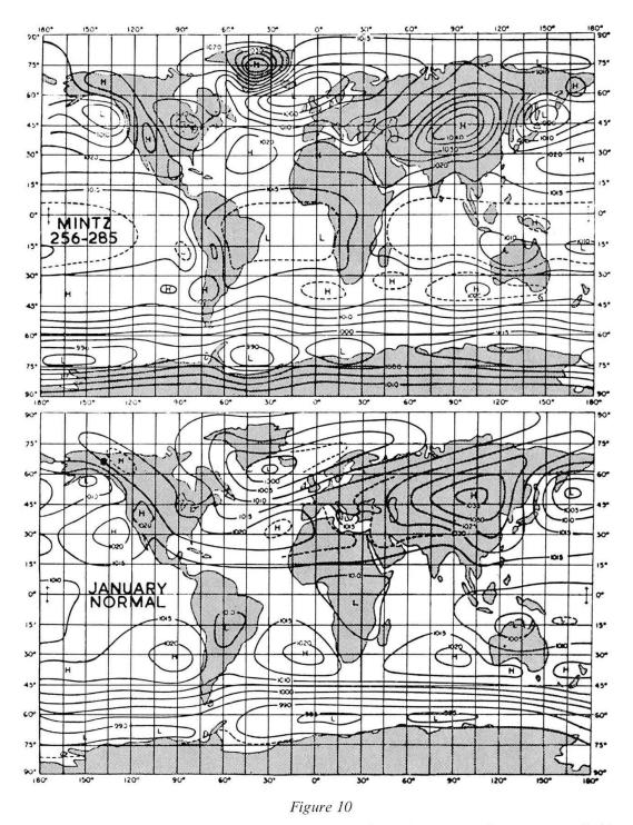
Comparison of computed (above) with observed (below) mean surface pressure (mb) for January. Note general agreement but presence of spurious anticyclone over Greenland in model atmosphere. (After MINTZ.)
