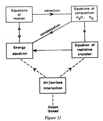
A schematic diagram showing the physics involved in an extended integration of the equations which determine the evolution of the atmosphere. Each box represents equations deriving from basic physical laws (of momentum, energy, etc.) and the interplay of one process with another is indicated by arrows between boxes. Not all operative interactions are shown.
