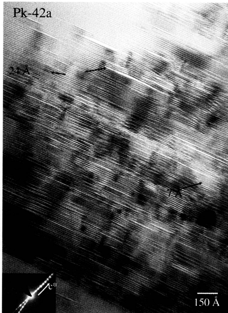
Fig. 6 Lattice-fringe image of chlorite crystals having lower periodicities (e.g. 7-Å), layer terminations (left arrow) and narrow voids affecting only one layer (e.g. right arrow). In the upper left 24-Å layers have been detected. The SAED, with 14-Å periodicity, shows streaking along c^* .
