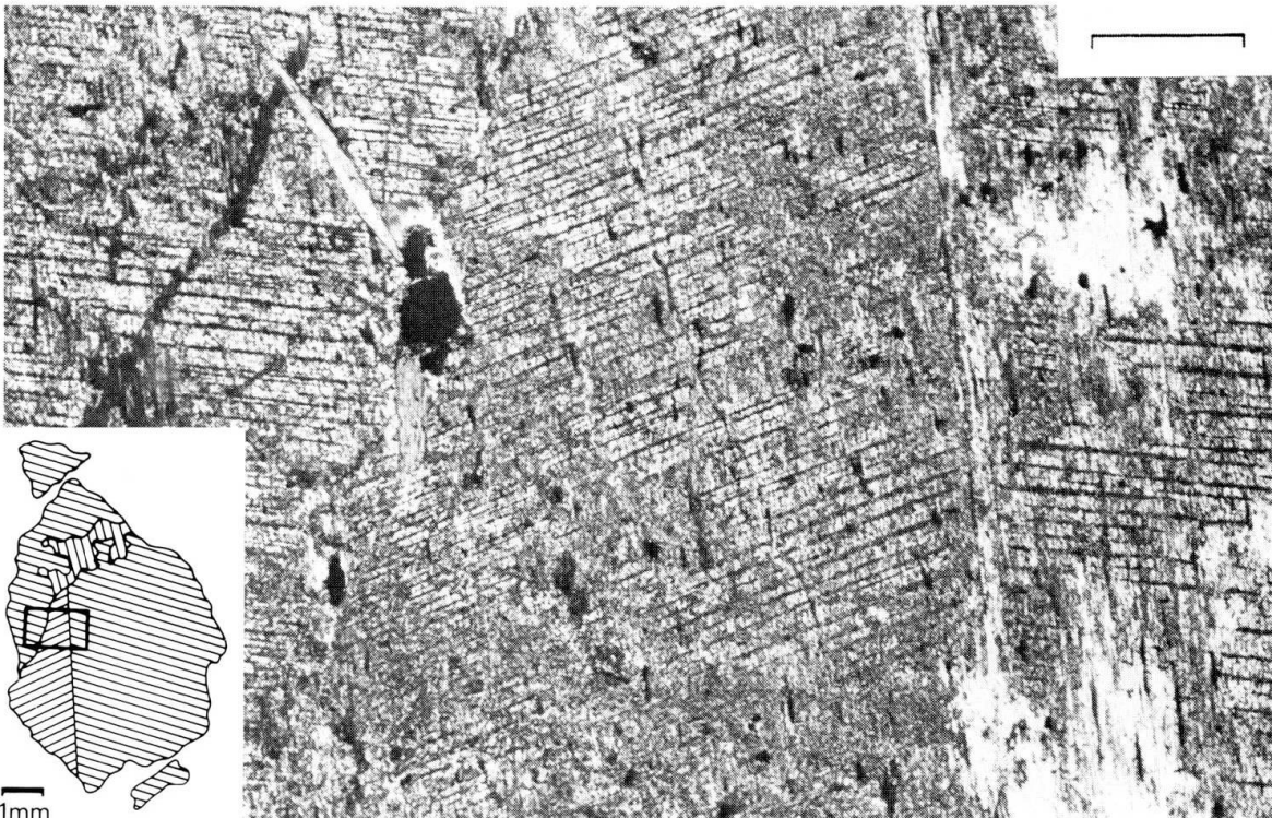
Fig. 4: Herringbone structure produced by the combination of (001) lamellae and a (100) twin in augite. The inset shows the relation between the twins, the rectangle represents the position of the micrograph. One twin is wedge-shaped and is surrounded by the other. The straight interface on the right is the (100) twinning plane, the left interface is irregular. At the point of the wedge-shaped twin another interlocking augite grain is visible. Crossed nicols, scale mark in the micrograph is 0,2 mm.
