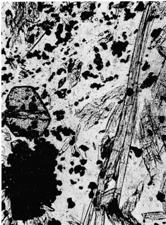
Fig. 3. Braunit (opak) - Spessartin (idiomorpher Kristall links) - Na-Amphibol (Prismen) Quarz-Albit (Matrix) - Fels. W Piz Corvatsch, S. Chastelets. Ohne Analysator.
