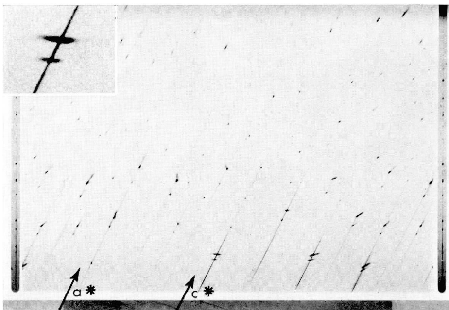
Fig. 5. Unmixed sanidine 2082. b -axis zero level Weissenberg photograph, calibrated according to PABST (1957). Unfiltered Cu radiation. The three monoclinic phases of this cryptoperthite are clearly visible. Three \beta^* values can be measured for each of the three distinct c^* -axes. The inset diagram shows an enlargement of the (002) reflection.
