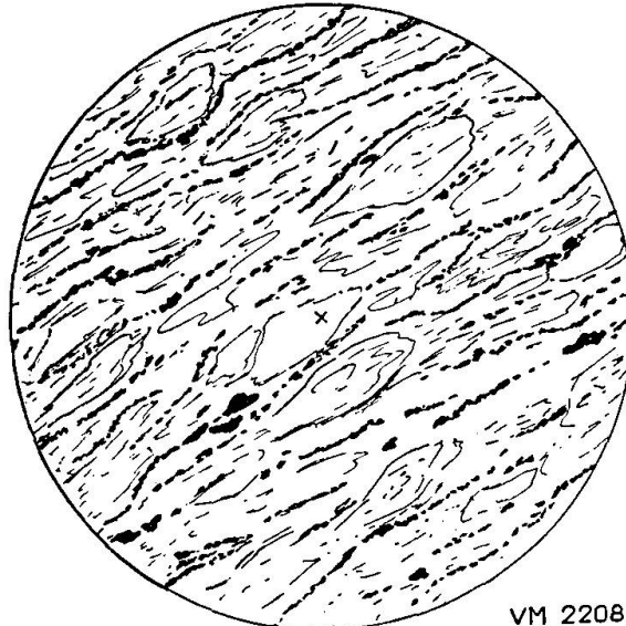
Fig. 4. Talc-magnetite schist. The Kangari Hills. Fine-grained magnetite, deposited around the flakes of talc and along the planes of schistosity. One Nicol.
