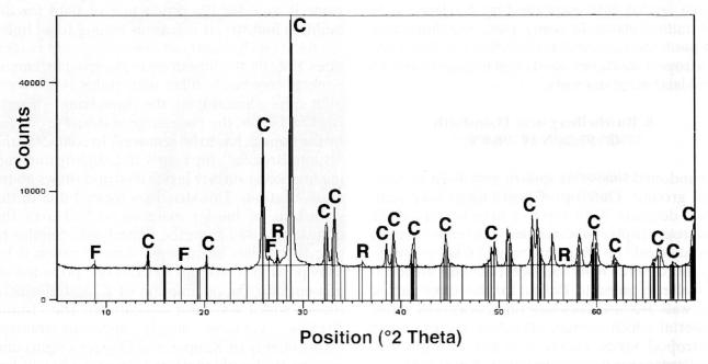
Fig. 2 X-ray diffractogram of HF-treated fraction  $<2 \,\mu m$  of white crystalline clast in suevite, collected during the excursion at Unterwilflingen/Ries. In addition to dominant coesite (C), minor rutile (R) and a fluoride (F) precipitated due to HF treatment are present.
