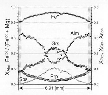
Fig. 8 Typical analytical transect of zoned garnet from metapelite (sample L005, 150 points) showing a continuous decrease in Fe<sup>tot</sup>/Fe<sup>tot</sup>+Mg ratio (Fe\*), indicative of a constant increase in T (prograde zonation). A slight increase in Mn-content at the very border is indicative of resorption (grey bands). However, the Fe\* ratio remains constant (or shows a slight decrease) in this border, indicative of constant (or a bit higher) T.
