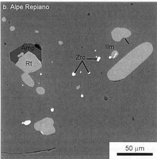
Fig. 12 (a) Photomicrograph of Alpe Repiano sample Rep9702. Garnet porphyroblasts are surrounded by a rim of granoblastic amphibole in a matrix of mostly clinopyroxene-plagioclase symplectite. (b) BSE image of inclusions of rutile and exsolved zircon in a 5 mm-sized garnet in Rep9702.
