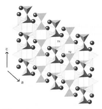
Fig. 1 Structural model of K-feldspar. A 3-dimensional framework of  $TO_4$  tetrahedra (depicted as polyhedra) creates cavities, which host the large alkali cations (drawn as spheres). T1 (stripe-filled) and T2 (rendered gray) designate the two symmetrically distinguishable T-sites. Si, Al and Fe are distributed between these two sites in K-feldspar from Itrongay.
