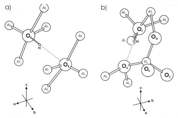
Fig. 7 Part of the kyanite crystal structure demonstrating the proposed OH defect incorporation model for (a) partial OH replacement of the  $O_B$  oxygen position, related to the band at 3386 cm<sup>-1</sup>, (b) partial OH replacement of the  $O_F$  oxygen position, related to the doublet band at 3275 and 3260 cm<sup>-1</sup>.
