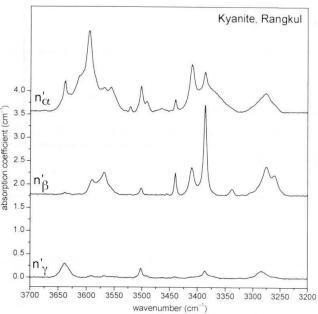
Fig. 3 Polarised OH absorption spectra of kyanites from Roberts Victor mine and Rangkul, recorded parallel to the  $n'_{\alpha}$ ,  $n'_{\beta}$  and  $n'_{\gamma}$  extinction directions on (100) crystal plates and on plates cut parallel to  $n'_{\gamma}$  and perpendicular to (100). Spectra are offset for clarity. The strong bands above 3500 cm<sup>-1</sup> in the sample from Rangkul are caused by submicroscopic hydrous mineral inclusions.
