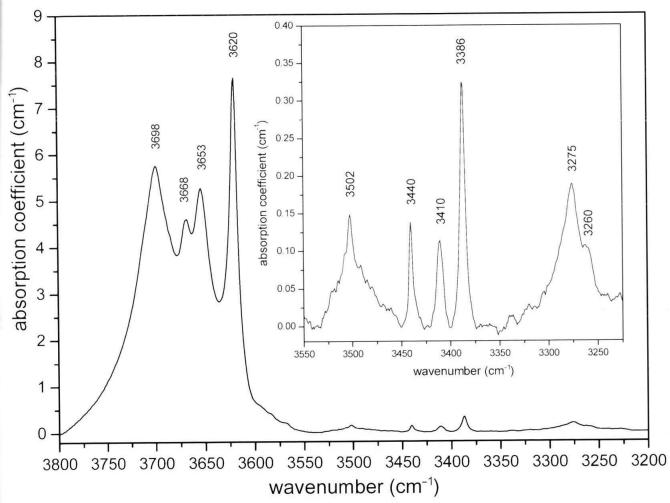
Fig. 2 Unpolarised IR spectrum in the OH stretching vibrational range of kyanite from Mangari, taken through turbid crystal parts. The strong OH absorption features in the 3600–3750 cm<sup>-1</sup> region correspond to those of kaolinite. The OH bands of the kyanite host are shown in the inset.
