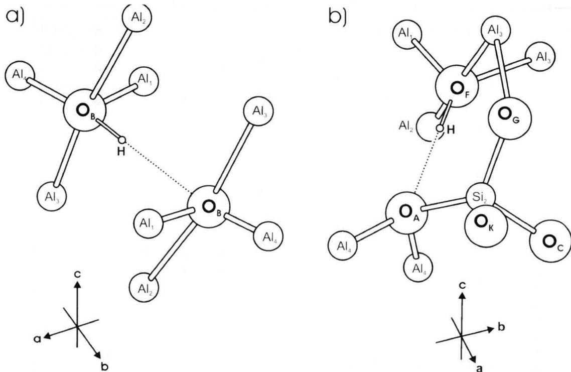
Fig. 7 Part of the kyanite crystal structure demonstrating the proposed OH defect incorporation model for (a) partial OH replacement of the  $O_B$  oxygen position, related to the band at  $3386\text{ cm}^{-1}$ , (b) partial OH replacement of the  $O_F$  oxygen position, related to the doublet band at  $3275$  and  $3260\text{ cm}^{-1}$ .
