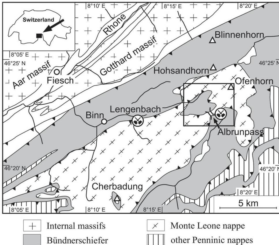
Fig. 1 Tectonic map of the larger Binn Valley area, Switzerland/Italy, where numerous base metal occurrences are associated with Triassic lithologies of the Monte Leone nappe (simplified after Spicher, 1988). The box marks the enlargement shown in Fig. 2.
