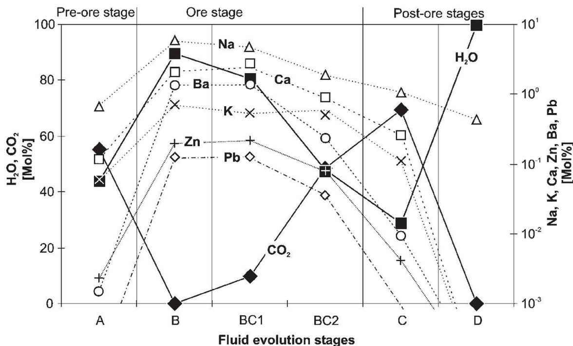
Fig. 7 Average molar concentrations of  $\text{H}_2\text{O}$  and  $\text{CO}_2$  (left, derived from microthermometry) and of Na, K, Ca, Zn, Ba and Pb (right, from LA-ICPMS) in the fluid plotted as a function of progressive fluid stages defined by petrography. Refer to Fig. 6 for the different fluid stages. Note the conspicuous increase of element concentrations with incursion of brine stage (B).
