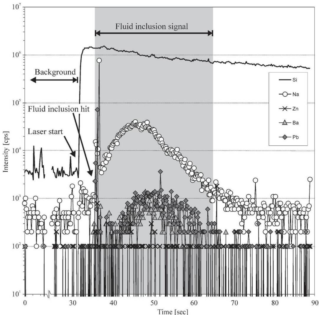
*Fig. 10* Transient LA-ICPMS signal of a CO<sub>2</sub>-rich inclusion with the typical spike at the time the inclusion is opened by the laser, corresponding to a sudden internal pressure release, followed by a smooth curve while the inclusion is ablated entirely.
