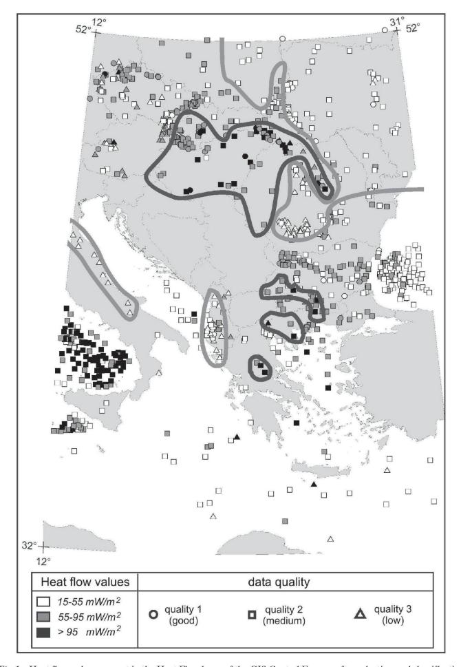
Fig. 1 Heat flow values present in the Heat Flow layer of the GIS Central Europe, after selection and classification among the available data (IHFC database and recently published values). Arbitrary contouring delineates areas of anomalously high and low heat flow values (dark gray and light gray contours respectively).
