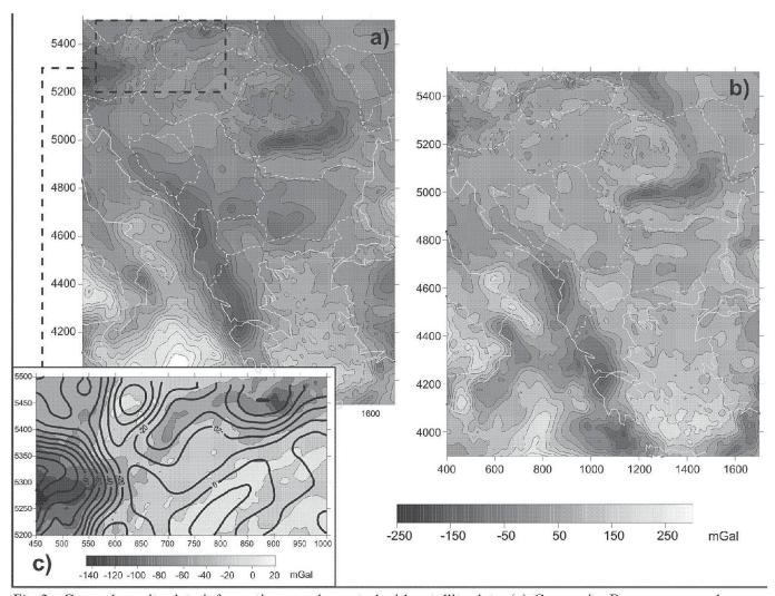
Fig. 2 Ground gravity data information supplemented with satellite data. (a) Composite Bouguer anomaly map. (b) Topo-isostatic anomaly map. (c) Comparison of the ground (underlying image) and satellite (overlying contours) Bouguer anomalies in a test zone.
