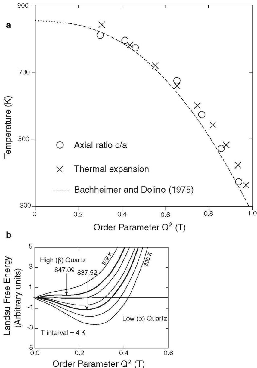
Fig. 5 The order parameter squared ( $Q^2$ ) as a function of Kelvin temperature (a) and Landau Free Energy (b). Our results for thermal expansion and the axial ratio  $c/a$  (Raz et al., 2002) are compared with the optical measurements of Bachheimer and Dolino (1975). The parabola  $e_1(T) = A' - A(1-T/T_0)^{1/2}$  with  $A = 0.01646$  fits the data for thermal expansion and the square of the Landau order parameter (Dolino and Bachheimer, 1984, Fig. 4)
