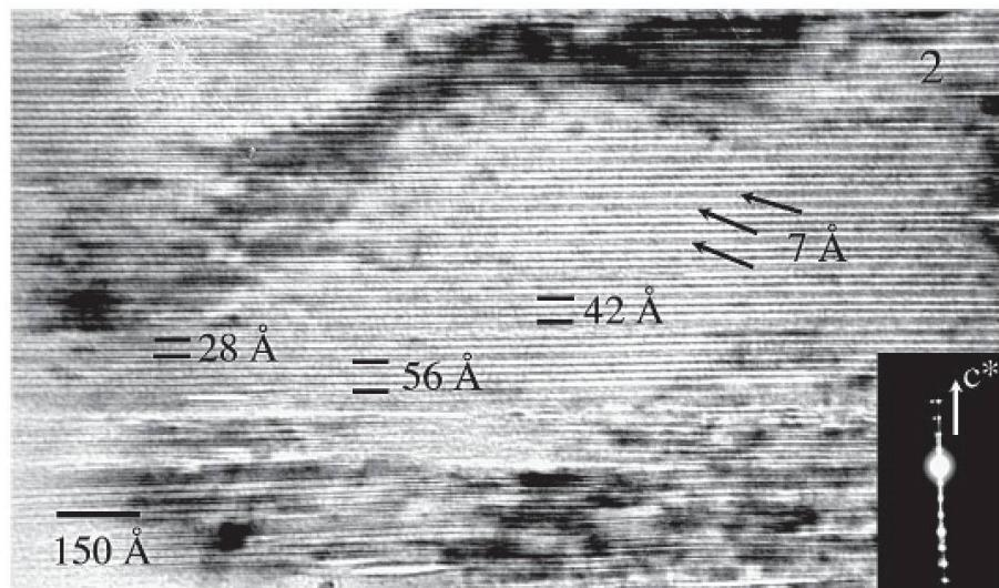
Fig. 4 Lattice-fringe image of a chlorite with fissures, contrast changes and distinct layer periodicities at 14 Å with alternating individual layers at 7 Å. Under SAED, the basal diffractions show dynamic effects produced by complex, multilayered polytypes at 14 Å.
