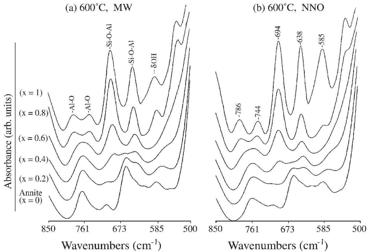
Fig. 5 Infrared spectra of micas along the annite-siderophyllite join in the range (850–500  $\text{cm}^{-1}$ ). (a) annite and Al-biotites obtained at 600 °C/MW and 100 MPa  $P_{\text{H}_2\text{O}}$ . (b) annite and Al-biotites obtained at 600 °C/NNO and 100 MPa  $P_{\text{H}_2\text{O}}$ .
