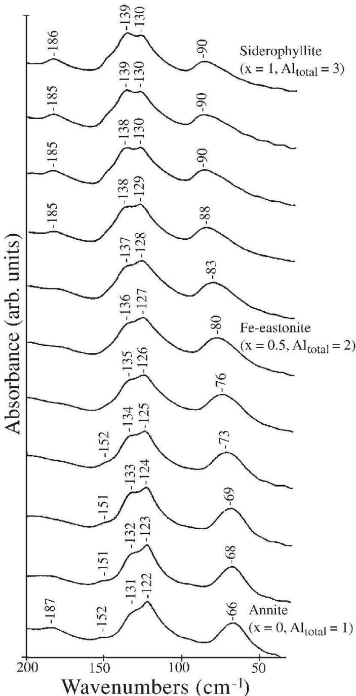
Fig. 1 Evolution of infrared spectra of annite compositions, along the annite-siderophyllite join in the frequency range of interlayer vibrations ( $200\text{--}50\text{ cm}^{-1}$ ).
