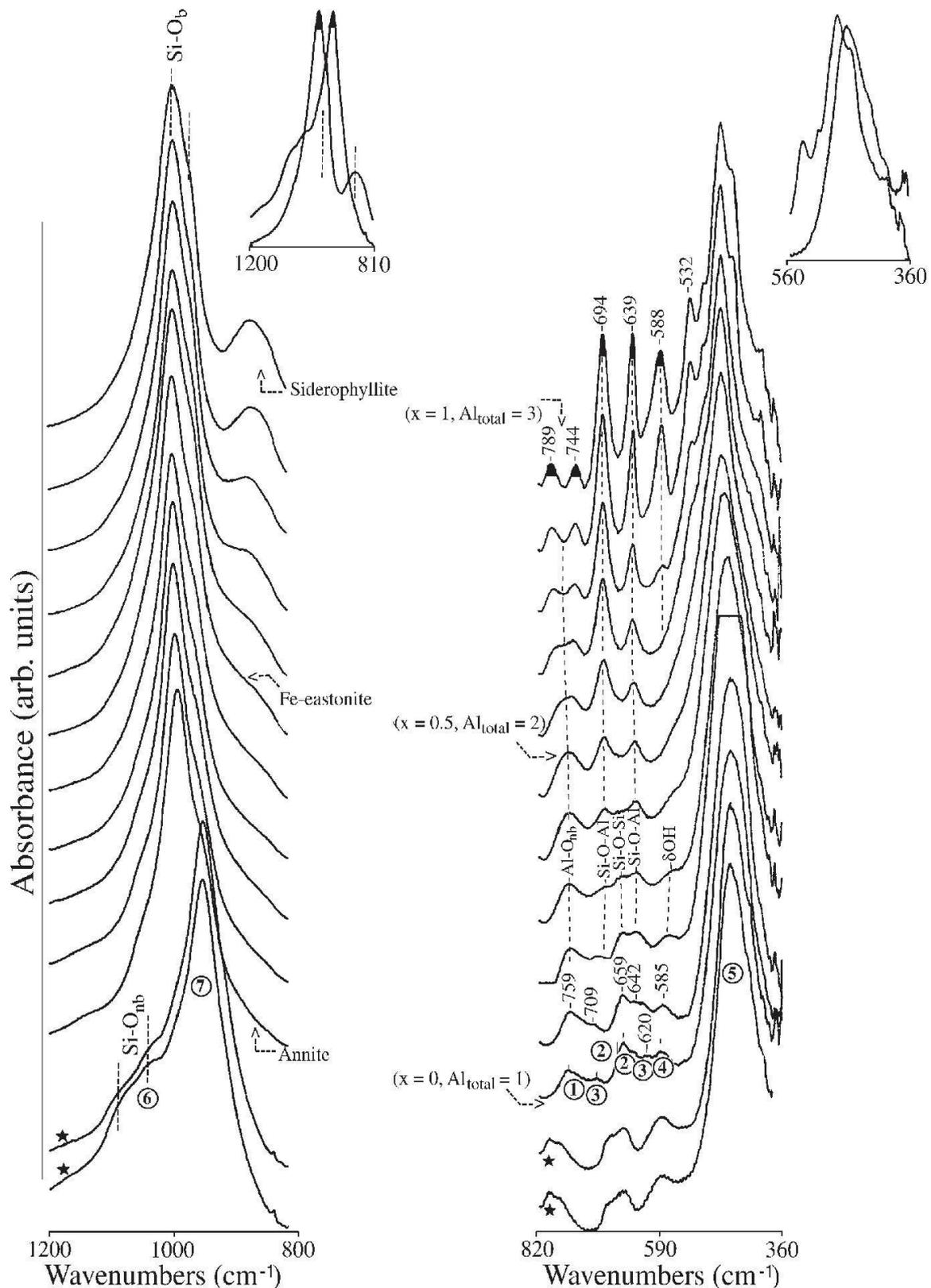
Fig. 3 Evolution of infrared spectra of annite compositions, along the annite-siderophyllite join and toward hypoaluminous iron compositions, in the frequency range of lattice vibrations (1200–800  $\text{cm}^{-1}$  and 820–360  $\text{cm}^{-1}$ ). Hypoaluminous iron compositions are denoted with stars.
