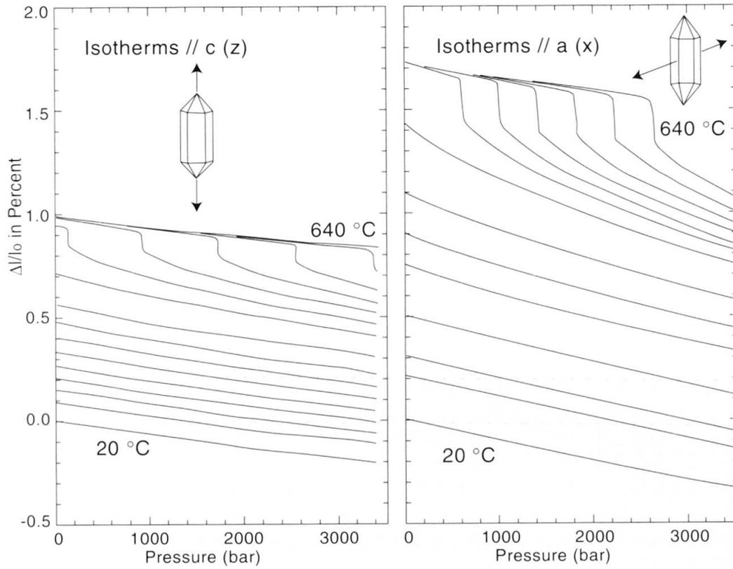
Fig. 4 Isothermal linear compressibility of quartz parallel to  $c(z)$  and  $a(x)$  axes at nominal temperatures between 20 °C and 640 °C. For precise temperatures and contour intervals see the corresponding Table 2 ( $//c(z)$  axis) and Table 3 ( $//a(x)$  axis).
