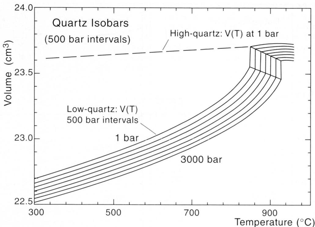
Fig. 6 Volumetric data for quartz as a function of temperature and pressure from 1 bar to 3 kbar (at 500 bar intervals). The volumetric data for high quartz has been extrapolated to lower temperatures, following the method of MAYER (1960), to determine ordering parameters.
