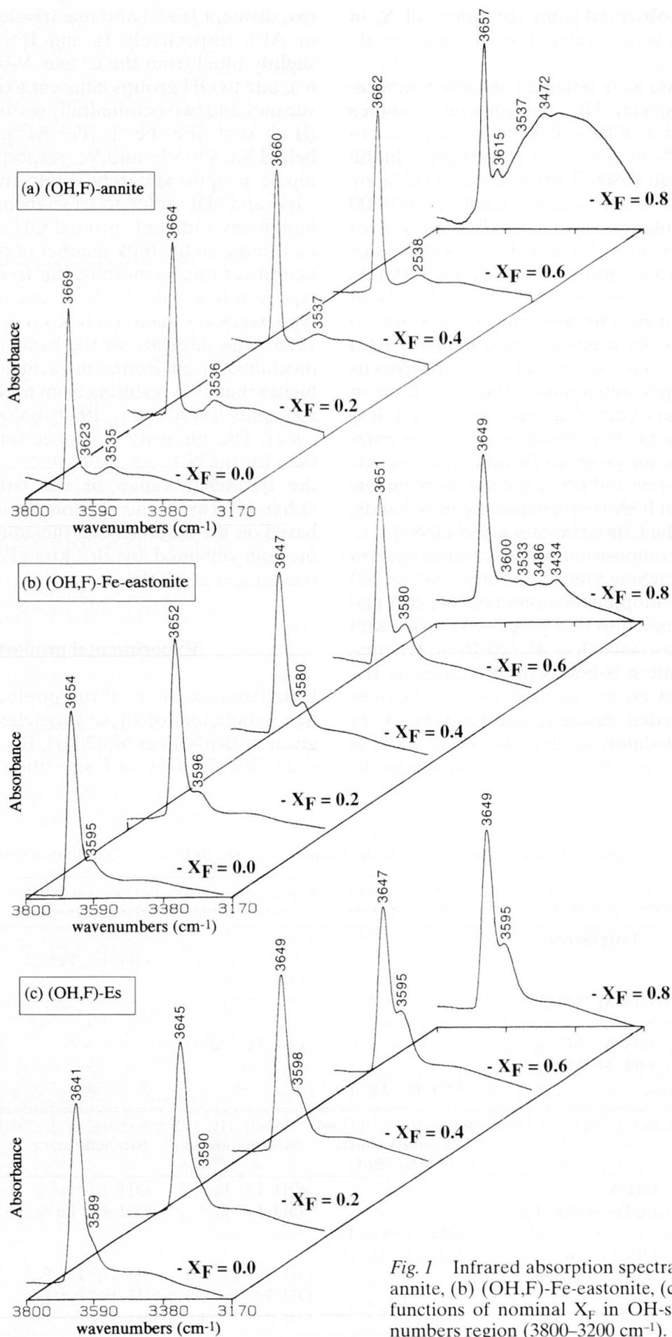
Fig. 1 Infrared absorption spectra of (a) (OH,F)-annite, (b) (OH,F)-Fe-eastonite, (c) (OH,F)-Es as functions of nominal  $X_F$  in OH-stretching wavenumbers region ( $3800\text{--}3200\text{ cm}^{-1}$ ).
