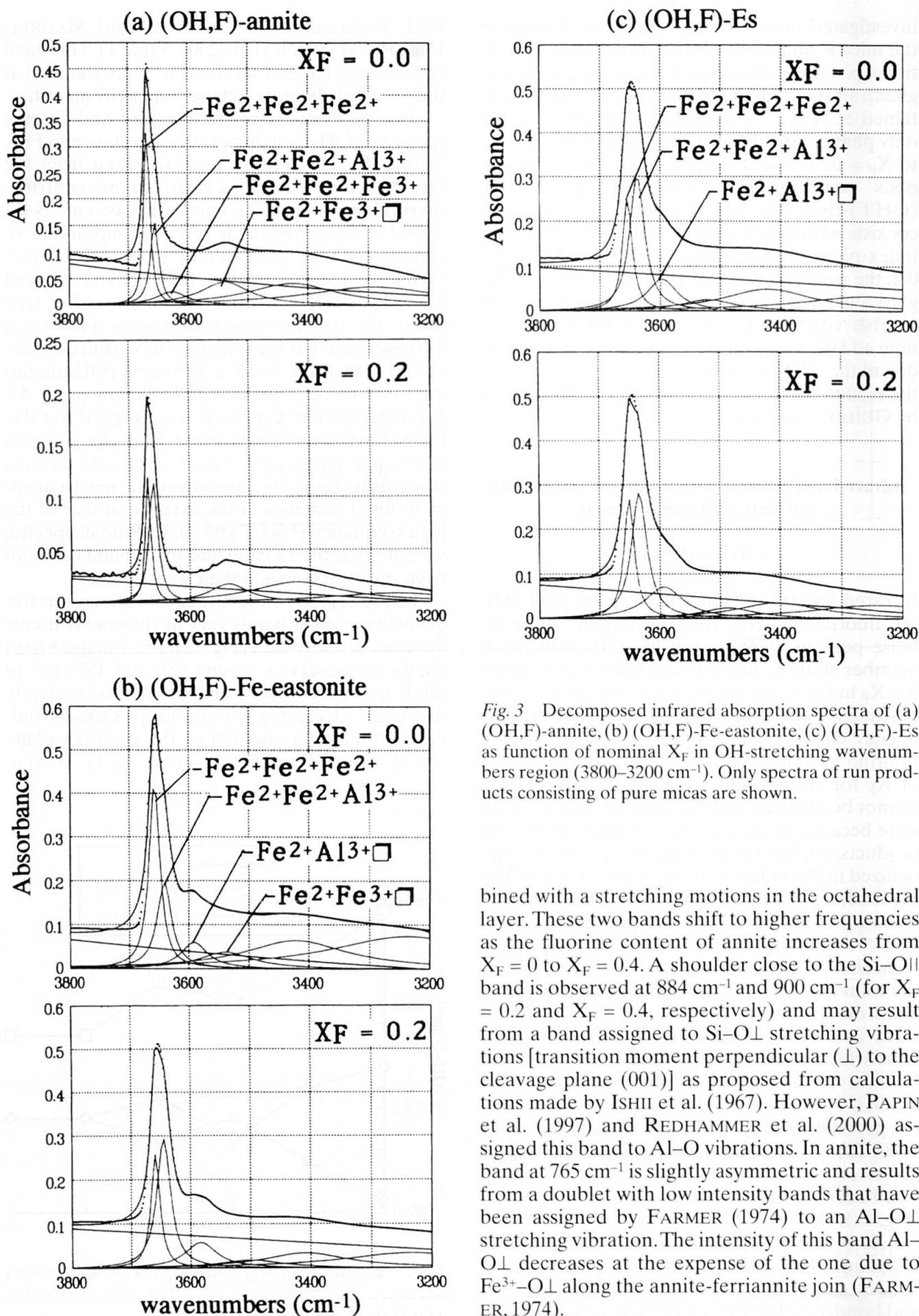
Fig. 3 Decomposed infrared absorption spectra of (a) (OH,F)-annite, (b) (OH,F)-Fe-eastonite, (c) (OH,F)-Es as function of nominal  $X_F$  in OH-stretching wavenumbers region (3800–3200  $\text{cm}^{-1}$ ). Only spectra of run products consisting of pure micas are shown.
