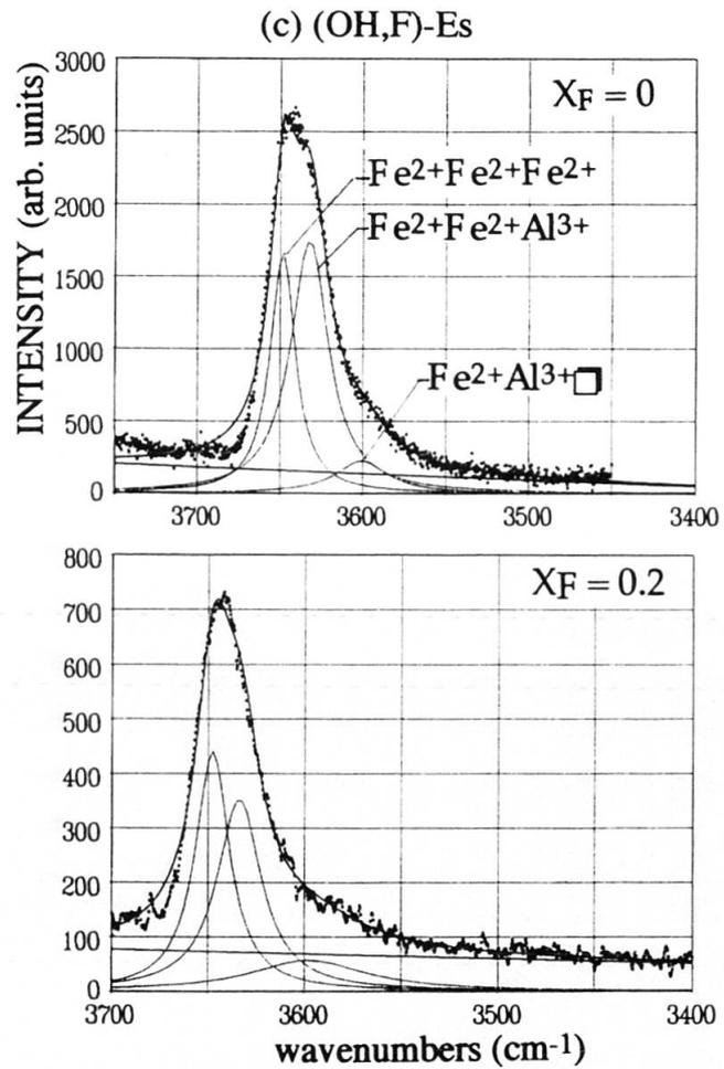
Fig. 4 Decomposed Raman scattering spectra of (a) (OH,F)-annite, (b) (OH,F)-Fe-eastonite, (c) (OH,F)-Es as function of nominal  $X_F$  in OH-stretching wavenumbers region (3800–3200 cm<sup>-1</sup>). Only spectra of run products consisting of pure micas are shown. The intensity scale is in total counts.
