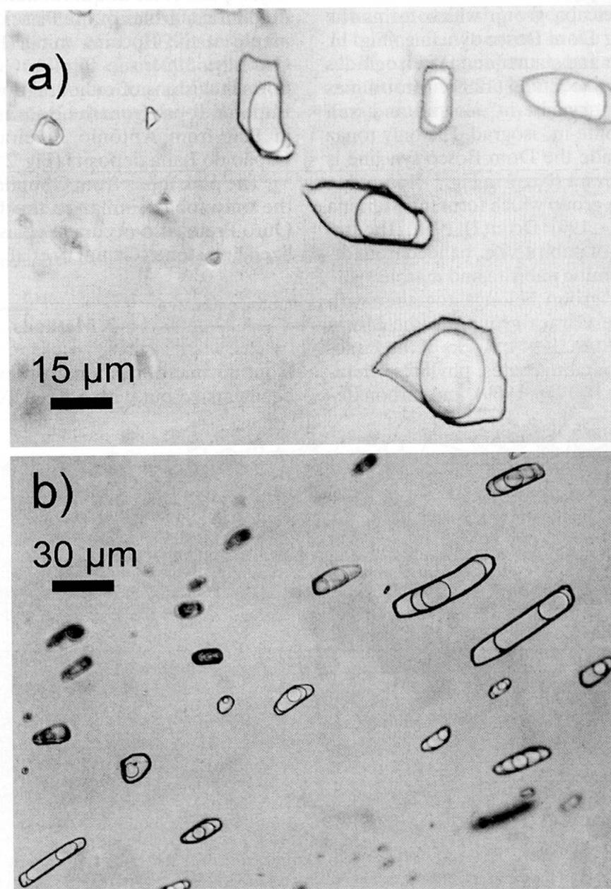
Fig. 3 Microphotograph showing typical 2-phase (a) fluid inclusions in Imperial Topaz from the deposit of Capão do Lana, and 3-phase (b) fluid inclusions in Imperial Topaz from the Dom Bosco deposit. Different gas/liquid ratios in the fluid inclusions suggest trapping below the solvus in the system  $H_2O/CO_2-NaCl$ . Due to very low  $CO_2$  contents, no liquid  $CO_2$  phase can be seen at room temperature in the inclusions of Capão do Lana.
