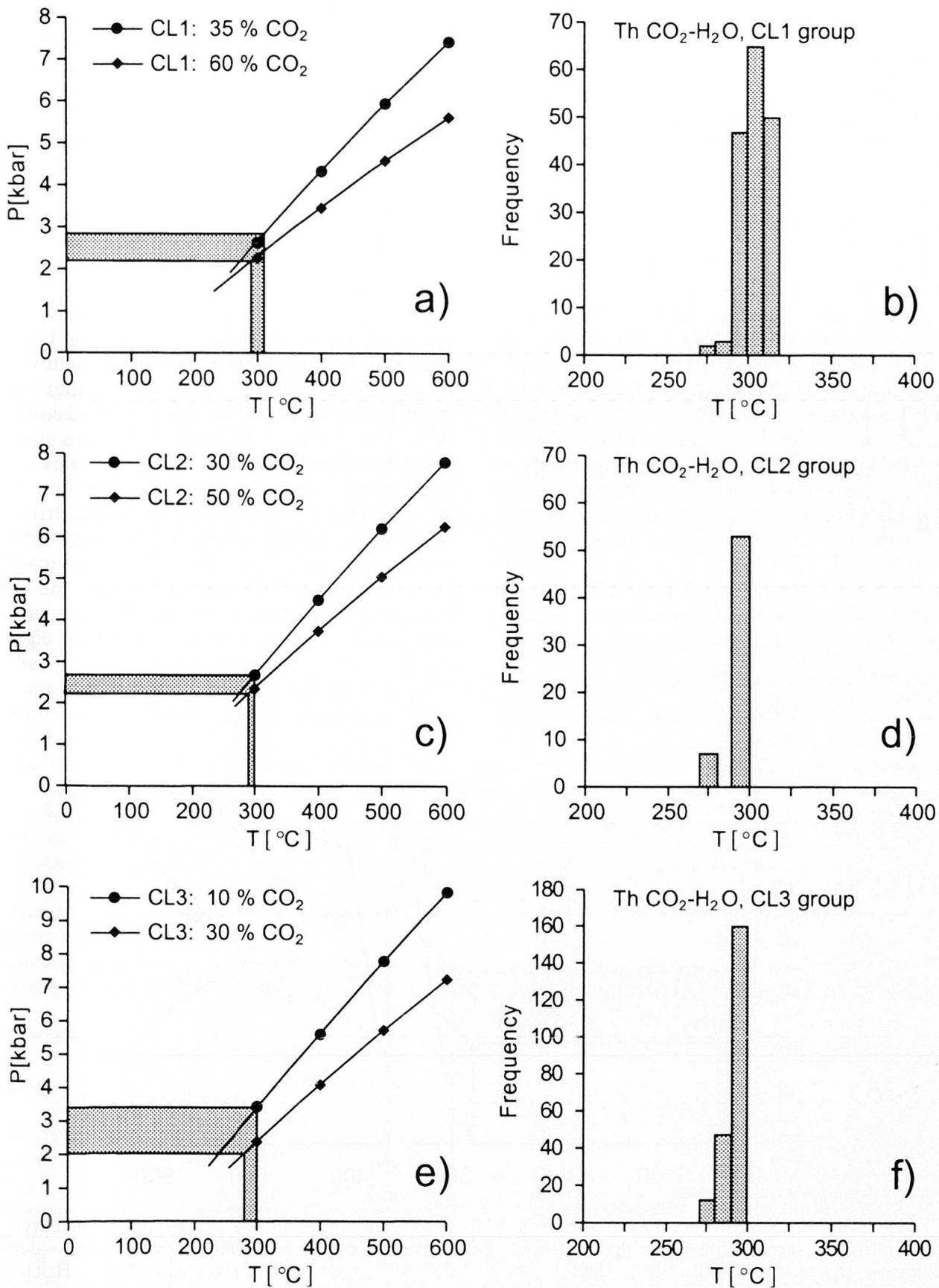
Fig. 4 (a, c, e): Isochores for fluid inclusions of topaz crystals of type CL1, CL2 and CL3, respectively. The isochores have been calculated with the FLINCOR<sup>®</sup> program package (BROWN, 1989) according to the equations of BOWERS and HELGESON (1983, 1985). The respective Th CO<sub>2</sub>-H<sub>2</sub>O temperatures are given in frequency diagrams (b, d, f).
