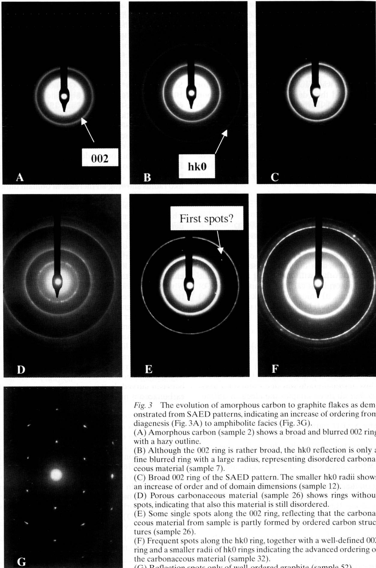
*Fig. 3* The evolution of amorphous carbon to graphite flakes as demonstrated from SAED patterns, indicating an increase of ordering from diagenesis (Fig. 3A) to amphibolite facies (Fig. 3G).
