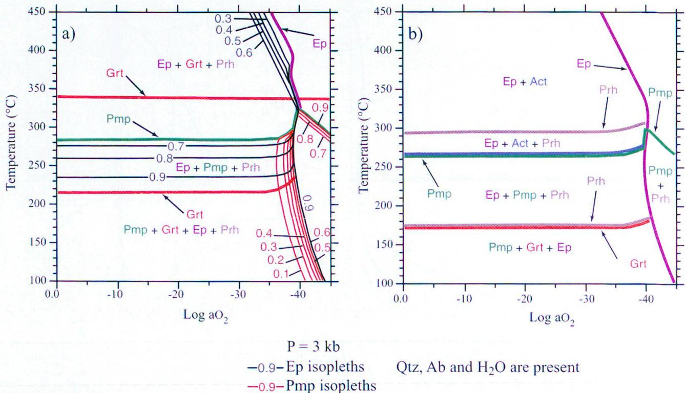
Fig. 12 T-Log  $a_{O_2}$  section at 3 kbar pressure in a HM-buffered system. The stability fields of the phases are drawn, and isopleths of pumpellyite and epidote are also plotted. Ep (epidote), Grt (garnet rich in Ca), Chl (chlorite) and Pmp (pumpellyite). (a) for rock composition of system 3; (b) for rock composition of system 3 with  $Mg/(Mg+Fe) = 0.26$ .
