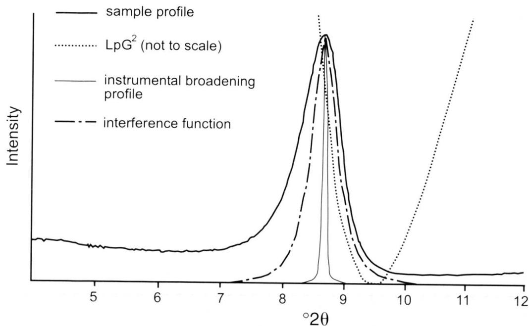
Fig. 1 Components of an X-ray diffraction peak (001 illite) used in calculating the X-ray scattering domain size. The sample profile shown is a Paleozoic mudstone from the Cantabrian zone of Spain.
