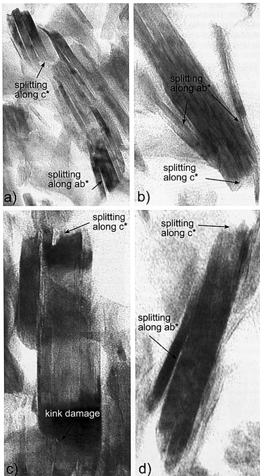
Fig. 8 Disaggregation damage of illite grains in pelites from SW England (SW samples documented in WARR and NIETO, 1998). Splitting of grains occurs along  $c^*$  and  $ab^*$ . (a) Diagenetic mudstones (SW1), (b) anchizonal slate, (c) anchizonal slate, (d) epizonal schist.
