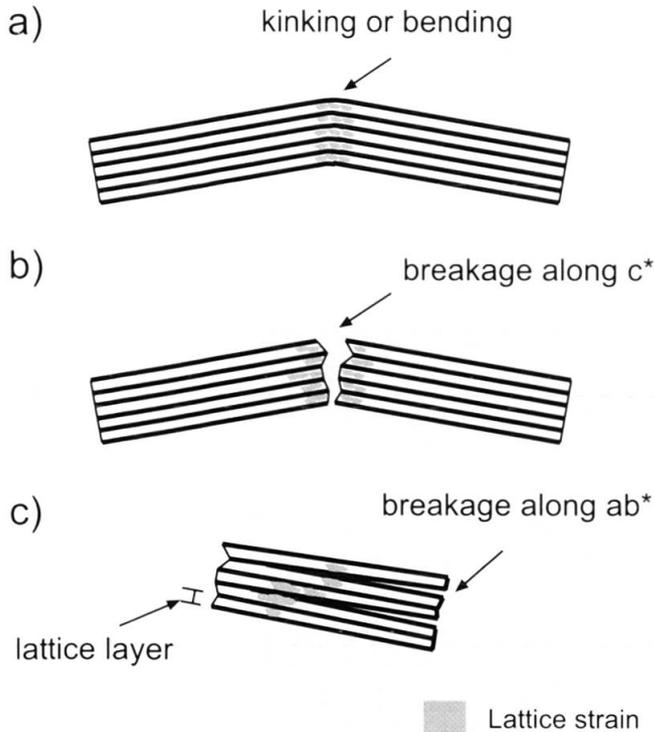
Fig. 6 Schematic diagram showing the various types of sample preparation damage caused by rock disaggregation (a) kinking or bending of crystals, (b) breakage roughly parallel to  $c^*$ , (c) breakage (splitting) along  $ab^*$ . Associated fields of lattice distortion (strained crystal) are also indicated.
