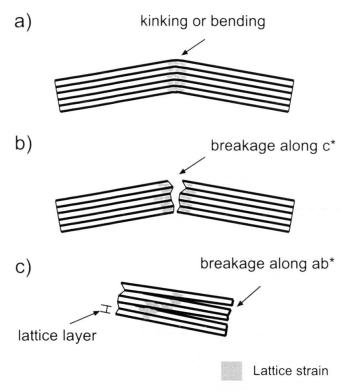
Fig. 6 Schematic diagram showing the various types of sample preparation damage caused by rock disagregation (a) kinking or bending of crystals, (b) breakage roughly parallel to c\*, (c) breakage (splitting) along ab\*. Associated fields of lattice distortion (strained crystal) are also indicated.
