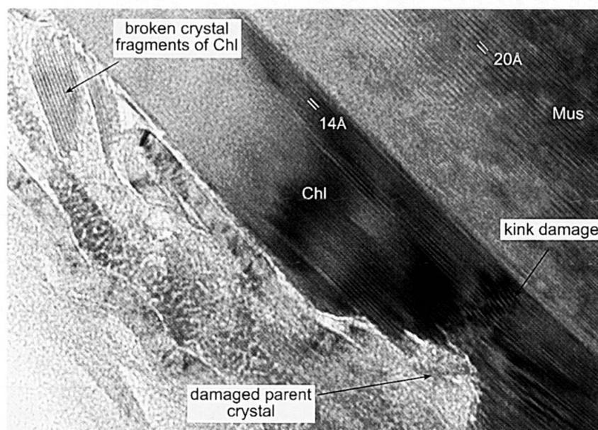
Fig. 7 Mechanical damage of a chlorite crystal in Otago Schist from New Zealand (Pumpellyite-actinolite facies) induced by initial dry grinding. Disaggregation damage occurs in the form of kink damage and broken fragments of chlorite that have been ripped-out of their parent chlorite crystals.
