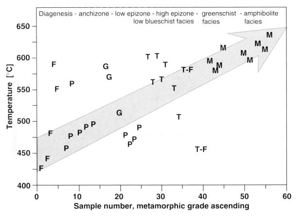
Fig. 8 Maximum temperatures of the DTA-TGA curves of organic matter (OM) concentrates, with oxygen as carrier gas. With increasing metamorphic grade, from left towards the right, maximum temperature increases. Code as in Fig. 7. Heterogeneities in OM composition causes a broad scatter at low metamorphic grade. Sample 40 containing migra-bituminite is strongly erratic.
