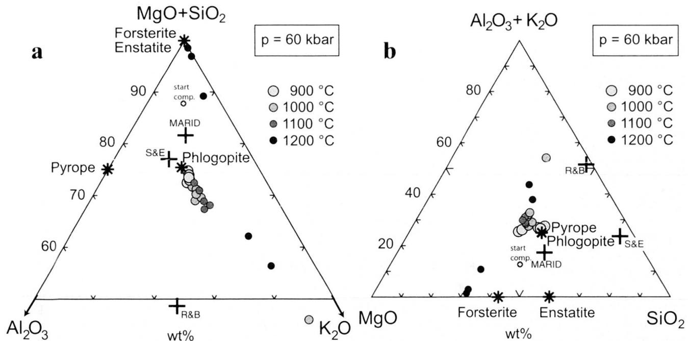
Fig. 2 Composition of the dry solute in the run series forsterite-phlogopite-H<sub>2</sub>O at 60 kbar: (a) MgO+SiO<sub>2</sub>-Al<sub>2</sub>O<sub>3</sub>-K<sub>2</sub>O ternary diagram (wt%) and (b) Al<sub>2</sub>O<sub>3</sub>+K<sub>2</sub>O-MgO-SiO<sub>2</sub> ternary diagram (wt%). For explanations see Fig. 1.
