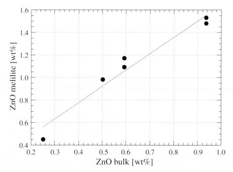
Fig. 7 Bulk ZnO concentration versus average ZnO concentrations in melilite. The linear regression equation is  $\text{ZnO}_{\text{mel}} = 1.45 \times \text{ZnO}_{\text{bulk}} + 0.2 \text{ (R}^2 = 0.95)$ . Analyses from 6 thin sections of 4 different samples.
