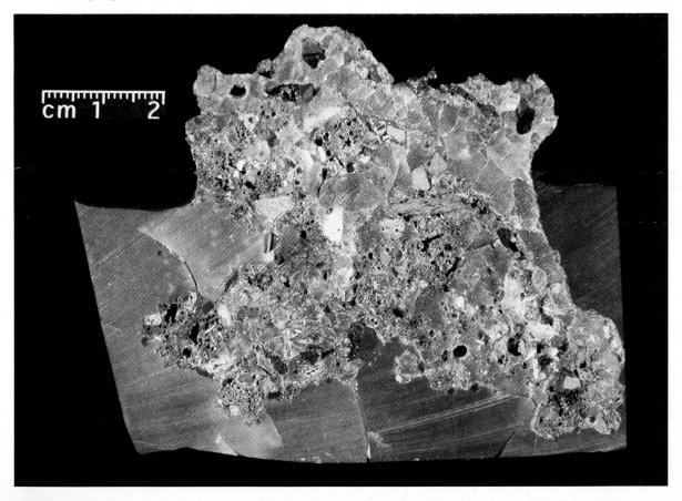
Fig. 22 Hand specimen of a heterogeneous slag embedded in resin (sample Kü6). Matrix consisting of newly formed glasss and of scrap glass with various refractory inclusions. Scale bar in [cm].
