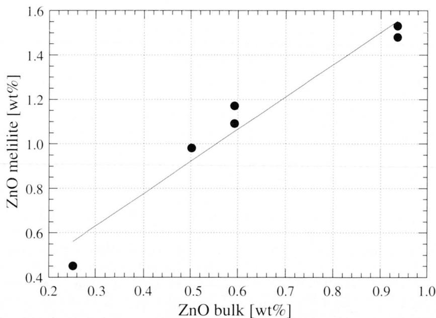
Fig. 7 Bulk ZnO concentration versus average ZnO concentrations in melilite. The linear regression equation is  $ZnO_{mel} = 1.45 \times ZnO_{bulk} + 0.2$  ( $R^2=0.95$ ). Analyses from 6 thin sections of 4 different samples.
