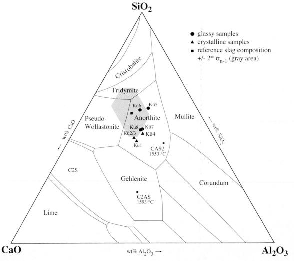
Fig. 5 Projection of bulk compositions into the melt system CaO-Al<sub>2</sub>O<sub>3</sub>-SiO<sub>2</sub> (redrawn form Levin, 1964) and comparison to reference bottom ash (grey area).
