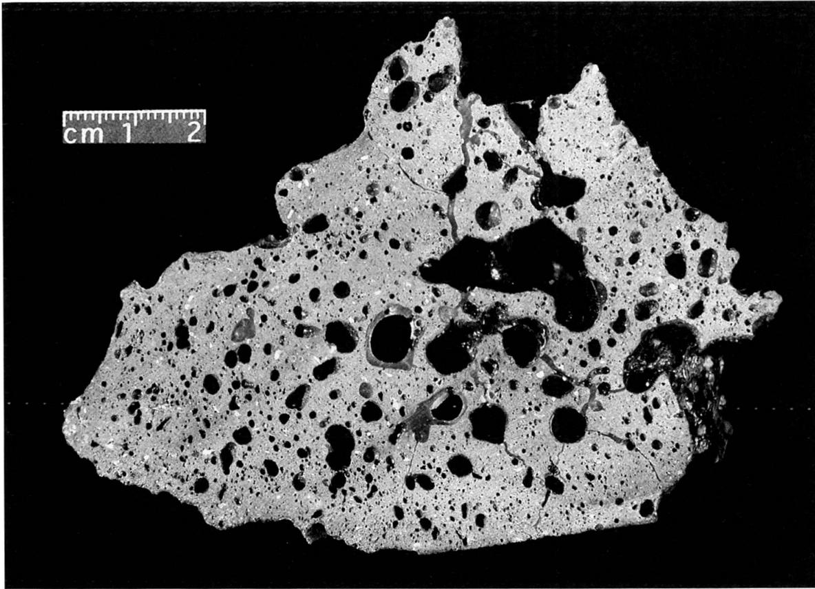
*Fig. 11* Hand specimen of a relatively homogeneous massive porous slag (sample Kü2). Pores are partly filled with resins. Scale bar in [cm].
