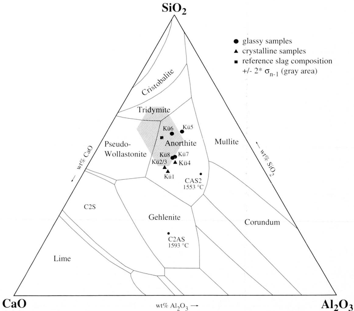
Fig. 5 Projection of bulk compositions into the melt system CaO–Al<sub>2</sub>O<sub>3</sub>–SiO<sub>2</sub> (redrawn from LEVIN, 1964) and comparison to reference bottom ash (grey area).
