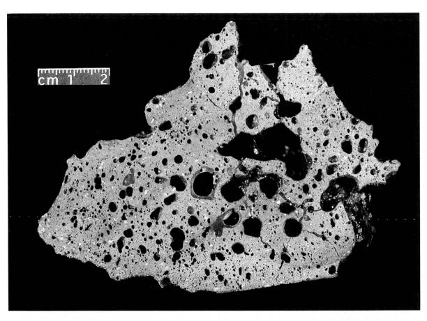
Fig. 11 Hand specimen of a relatively homogeneous massive porous slag (sample Kü2). Pores are partly filled with resina. Scale bar in [cm].
