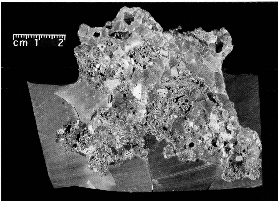
*Fig. 22* Hand specimen of a heterogeneous slag embedded in resin (sample Kü6). Matrix consisting of newly formed glass and of scrap glass with various refractory inclusions. Scale bar in [cm].
