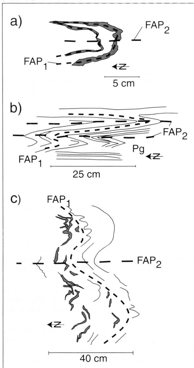
Fig. 5 Deformation style during  $D_2$  and  $D_3$  as observed within amphibolites, metapelites and paragneisses with relict structures of older deformation phases ( $D_1$ ). a)  $D_2$ -fold in a paragneiss of the Simano nappe. b)  $D_2$ -folds in a metapelite of the Adula nappe. c)  $D_3$ -folds as found in both nappes. Note that the folding style occurs at all scales.
