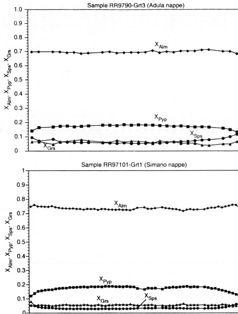
Fig. 7 Garnet profiles measured with the electron microprobe in samples RR97-90 (Adula nappe, 30 measurement points with a spacing of 21 $\mu$ m) and RR97-101 (Simano nappe, 60 measurement points with a spacing of 41 $\mu$ m). The left and right edges of the diagram correspond to the rim of the garnet.
