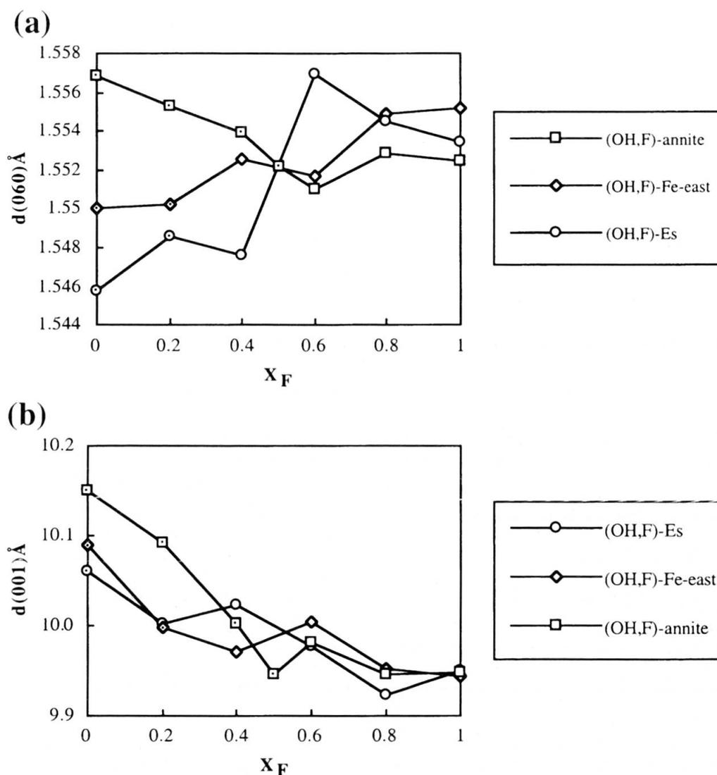
Fig. 1 Variations of measured interplanar distances  $d_{060}$  and  $d_{001}$  (in Å)  $\pm 0.0004$  versus nominal fluorine content ( $X_F$ ) of the studied micas. Dotted symbols denote samples composed of mica only.
