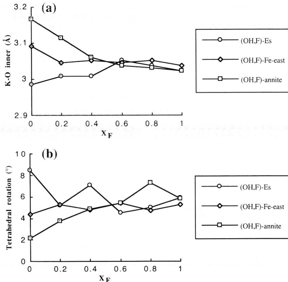
Fig. 6 (a) Variation of calculated K-O<sub>inner</sub> distance versus nominal fluorine content of the micas studied. O<sub>inner</sub>: inner oxygens, which are close to the interlayer cation (TATEYAMA et al., 1977). (b) Relationship between calculated tetrahedral rotation angles and X<sub>F</sub>. Tetrahedral rotation angles ( $\alpha_2$ ) are calculated from the relation proposed by TATEYAMA et al. (1977). Dotted symbols denote samples composed of mica only.
