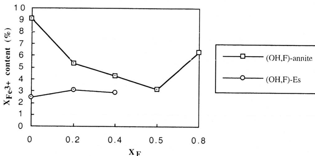
Fig. 2 Relationship between  $X_{\text{Fe}^{3+}}$  ( $= \text{Fe}^{3+}/\text{Fe}_{\text{total}}$ ) content (in %) obtained from Mössbauer measurements versus nominal  $X_{\text{F}}$ . Dotted symbols denote samples composed of mica only.
