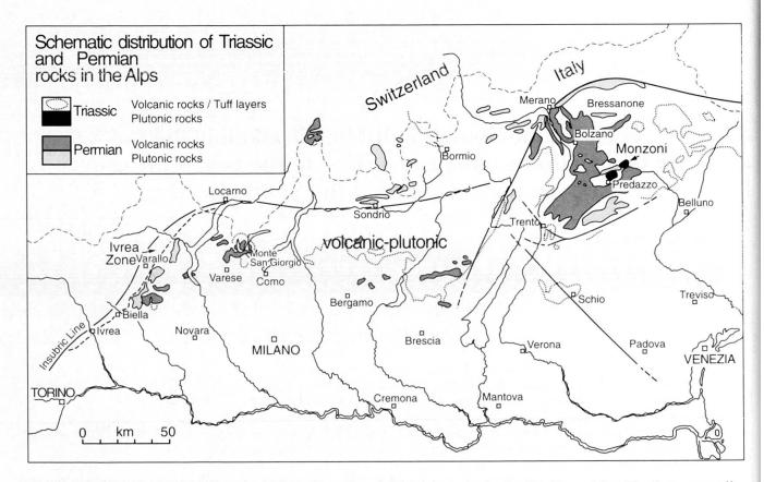
Fig. 1 Distribution of the Triassic and Permian volcanic/plutonic rocks in the Southern Alps. The Ivrea zone lies southeast of the Insubric Line at the western termination of the Southern-Alpine region (after FIORENTINI POTENZA et al., 1975). The Lower Permian metagabbroic/metabasaltic rocks of the Ivrea zone are shown in figure 2.
