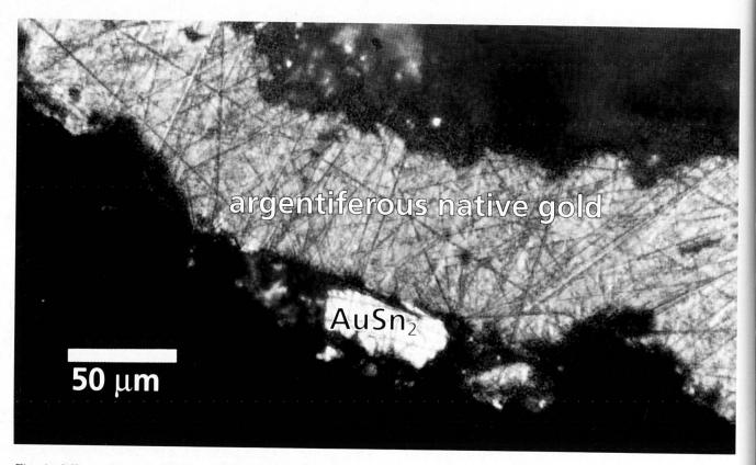
Fig. 4 Microphotograph of a AuSn<sub>2</sub> grain at the rim of an argentiferous native gold particle. Le Boiron river near Yens, canton Vaud. Partially crossed nicols; oil immersion.
