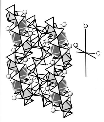
Fig. 1 Polyhedral drawing of the babingtonite structure displaying corrugated Fünfer-einfachketten extending parallel to the b-axis. Fe1 octahedra, predominantly occupied by divalent atoms (Fe, Mn, Mg), are dark gray with light rims and form edge-sharing doublets. Fe2 octahedra, predominantly occupied by trivalent atoms (Fe, Al), are light gray with black rims. Ca polyhedra are shown as spheres with bonds.
