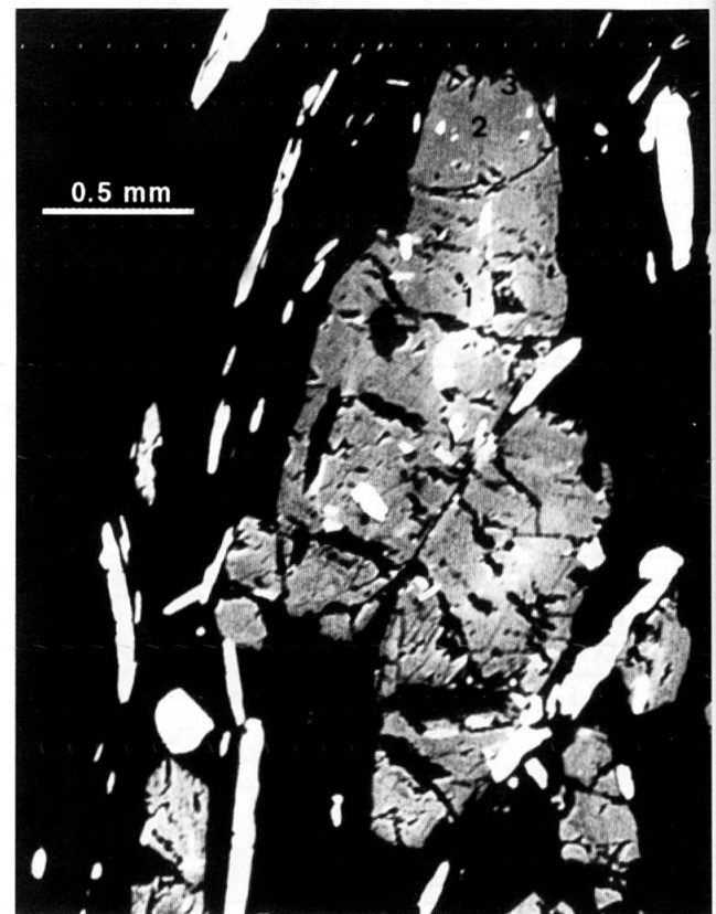
Fig. 5 Back scattered electron image of piemontite from the talc-free piemontite-quartz schist showing three zones: 1 = core with enrichment of Mn 3+ -content, 2 = mantle with depletion in Mn 3+ -content, and 3 = rim with enrichment in Mn 3+ -content.
