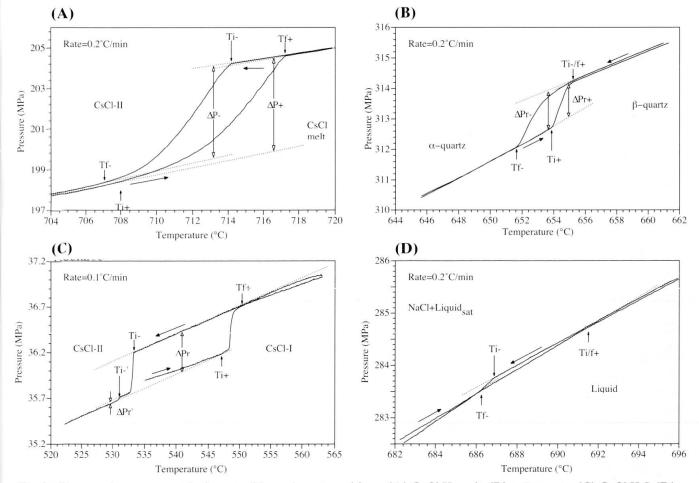
Fig. 3 Reversed pressure analysis runs of four phase transitions: (A) CsCl II-melt, (B)  $\alpha$ -β quartz, (C) CsCl II-I, (D) NaCl-liquidus. Arrows indicate heating (+), and cooling (–) runs. Heating and cooling rates are 0.1 or 0.2 °C/min. The pressure signals show different peak characteristics depending on the type of reaction. See text for details.
