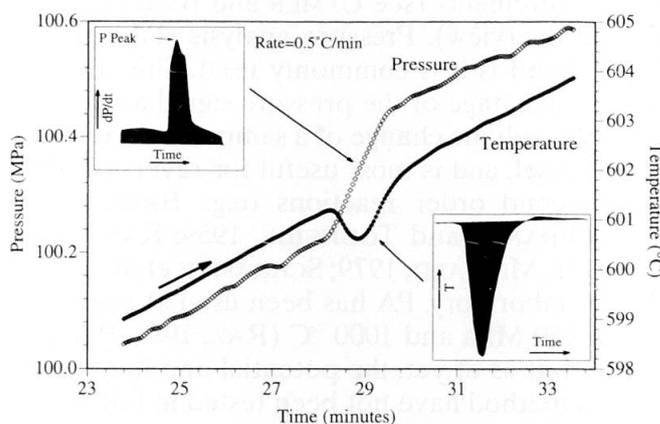
Fig. 2 Simultaneous pressure and temperature analysis of the  $\alpha$ - $\beta$  quartz transition. The reaction is endothermic and shows a positive  $\Delta V$ . The differential pressure and temperature signals are shown in insets. Maximum gradients in the T and P curves occur at the same time and most likely indicate maximum reaction progress.
