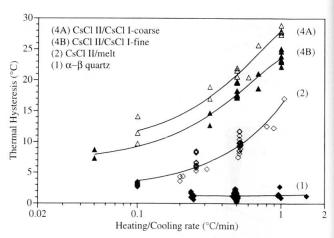
Fig. 6 Rate dependence of the thermal hysteresis of four reactions: the thermal hysteresis of the CsCl reactions shows a strong decrease with decreasing scan rates. The hysteresis of the  $\alpha$ - $\beta$  quartz reaction, on the other hand, was much smaller (1 °C) and quite insensitive for the chosen rates (see text for details).
