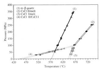
Fig. 4 Phase diagram (P-T) of the CsCl system and the  $\alpha$ -β quartz transition up to 750 °C and 350 MPa derived from PA data. Data points for heating and cooling runs are shown separately and can be fitted by straight lines. The thermal hysteresis for the CsCl reactions is larger than for the quartz reaction. The average fit equations are listed in table 1.
