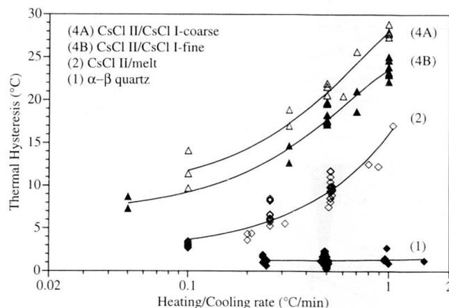
Fig. 6 Rate dependence of the thermal hysteresis of four reactions: the thermal hysteresis of the CsCl reactions shows a strong decrease with decreasing scan rates. The hysteresis of the  $\alpha$ - $\beta$  quartz reaction, on the other hand, was much smaller (1 °C) and quite insensitive for the chosen rates (see text for details).
