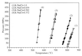
Fig. 5 Phase diagram (P-T) for the NaCl– $H_2O$  liquidus reaction. Curves are shown for different NaCl contents ( $X_{\text{NaCl}} = 1$  to  $X_{\text{NaCl}} = 0.37$ ). The equilibrium curves of reversed PA runs (rates = 0.5–0.1 °C/min) are increasingly steeper for lower salt contents.
