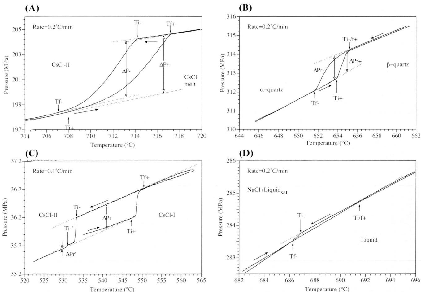
Fig. 3 Reversed pressure analysis runs of four phase transitions: (A) CsCl II-melt, (B)  $\alpha$ - $\beta$  quartz, (C) CsCl II-I, (D) NaCl-liquidus. Arrows indicate heating (+), and cooling (-) runs. Heating and cooling rates are 0.1 or 0.2 °C/min. The pressure signals show different peak characteristics depending on the type of reaction. See text for details.
