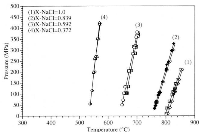
Fig. 5 Phase diagram (P-T) for the NaCl-H<sub>2</sub>O liquidus reaction. Curves are shown for different NaCl contents ( $X_{\text{NaCl}} = 1$  to  $X_{\text{NaCl}} = 0.37$ ). The equilibrium curves of reversed PA runs (rates = 0.5–0.1 °C/min) are increasingly steeper for lower salt contents.
