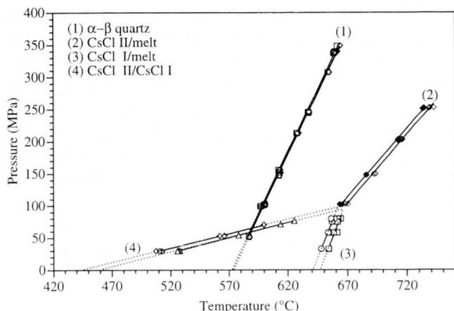
Fig. 4 Phase diagram (P-T) of the CsCl system and the  $\alpha$ - $\beta$  quartz transition up to 750 °C and 350 MPa derived from PA data. Data points for heating and cooling runs are shown separately and can be fitted by straight lines. The thermal hysteresis for the CsCl reactions is larger than for the quartz reaction. The average fit equations are listed in table 1.
