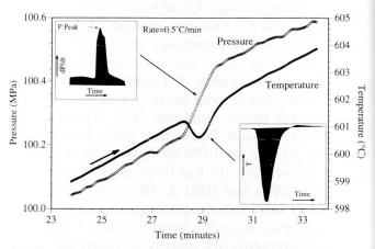
Fig. 2 Simultaneous pressure and temperature analysis of the  $\alpha$ - $\beta$  quartz transition. The reaction is endothermic and shows a positive  $\Delta V$ . The differential pressure and temperature signals are shown in insets. Maximum gradients in the T and P curves occur at the same time and most likely indicate maximum reaction progress.
