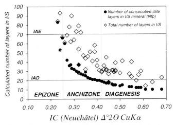
Fig. 6 Interpretation of the Neuchâtel IC scale (anchizone limits of 0.25° and 0.42° Δ2θ CuKα, based on the data of the PMR, interpreted with the method outlined here (see text for explanation). IAE: interpreted anchizone – epizone limit ( $N_{FP}=70$ ), IAD: interpreted anchizone – diagenesis limit ( $N_{FP}=20$ ).
