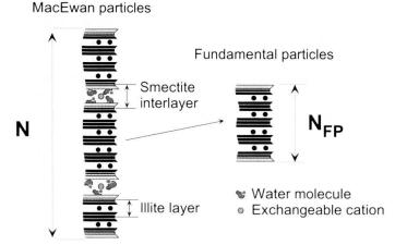
Fig. 4 I/S mixed-layers (= MacEwan particles) with high illite content can be considered as a stack of N illite layers joined by smectite interlayers. These illite stacks are the fundamental particles of NADEAU et al. (1984).
