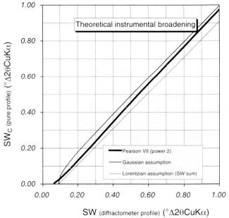
Fig. 2 Relation used to remove the instrumental broadening effect from the SW to obtain the Scherrer width of the pure profile (SW<sub>c</sub>). This net is created by the convolution of the instrumental profile with a Pearson VII (power 2) function used as pure profile. It is compared to the relationship obtained assuming Gaussian or Lorentzian profile for both instrumental and pure profiles.
