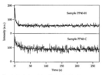
Fig. 4 Evolution of the CL-signal of the blue component at 2.76 eV. Experimental curves grey; curve fitting black. The fitting equation was:  $I(t) = B_L + I_1*exp(-t/T_1) + I_2*exp(-t/T_2)$  where  $B_L$ ,  $I_1$ ,  $I_2$ ,  $T_1$  and  $T_2$  are the fitting parameters.
