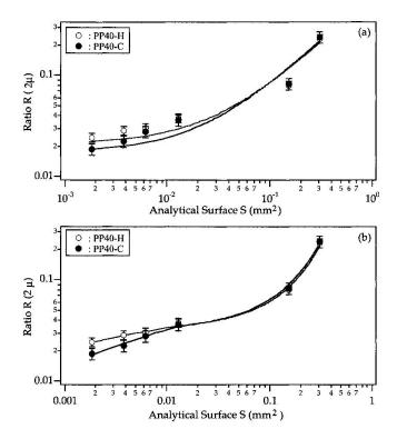
Fig. 5 Ratio R as a function of the analytical surface S. Both axis are in a logarithmic scale and the error bars for R are given in  $2\sigma$ . The thin curve is for PP40-C, the thick curve is for PP40-H. (a) fit function:  $f(x) = K_0 + K_1 \cdot \exp(-K_2 \cdot x)$ . (b) fit function:  $f(x) = \exp[K_0 + K_1 \cdot \exp(-K_2 \cdot x)] + K_3 \cdot \exp(-K_4 \cdot x)$  where the  $K_i$  are the fitting parameters.
