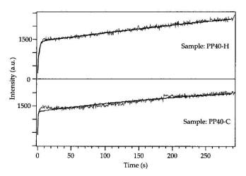
Fig. 3 Evolution of the CL-signal of the red component at 1.88 eV. Experimental curves grey; curve fitting black. The fitting equation was:  $I(t) = B_L - I_1 \cdot \exp(-t/T_1) - I_3 \cdot \exp(-t/T_2)$  where  $B_L$ ,  $I_1$ ,  $I_2$ ,  $I_1$  and  $I_2$  are the fitting parameters.
