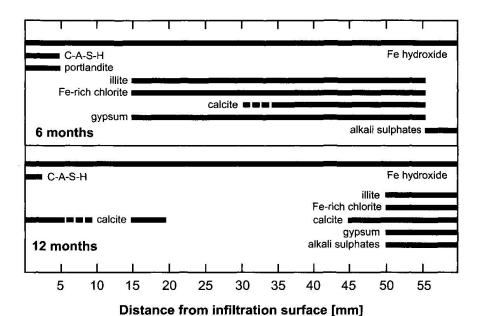
Fig. 4 Comparison of distribution of secondary minerals that formed in the advection experiments at different time steps. The right boundary of the graph represents the position of the evaporation surface of the rock sample. Dashed bars indicate uncertain identification of a mineral phase. See text for details. C-A-S-H: Ca-Al-Si-hydrate phase.
