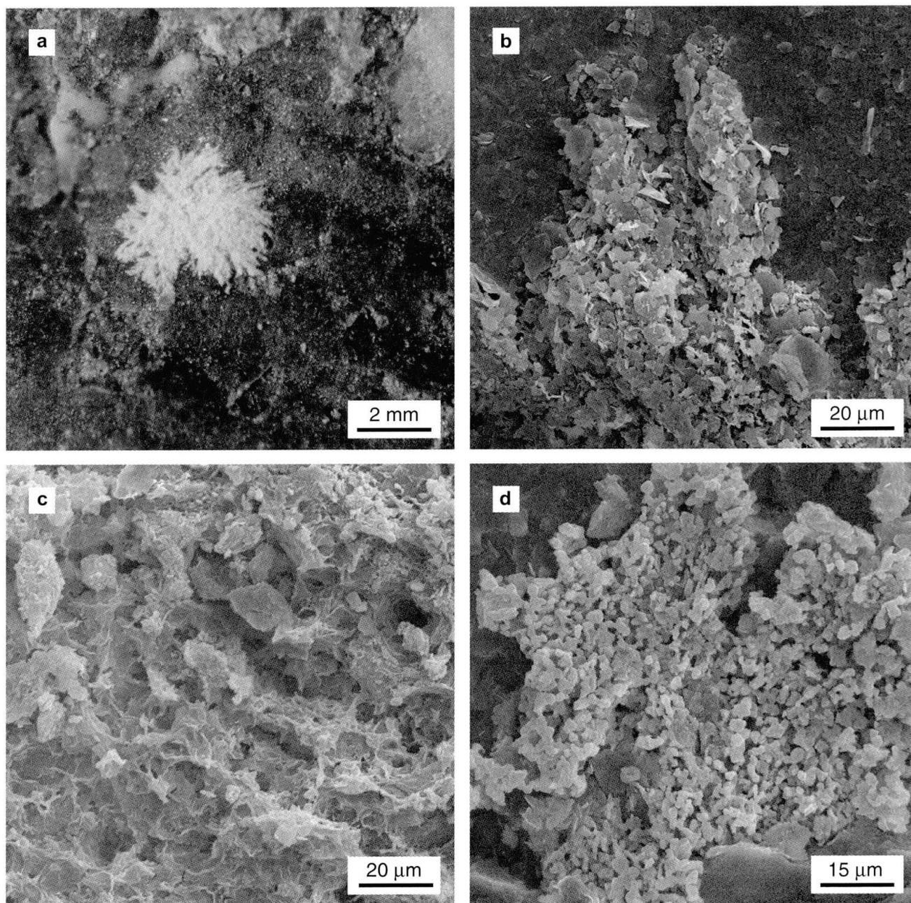
*Fig. 6* Photographs of secondary minerals in the advection experiments. (a) binocular microscopic image of new clay mineral assemblage (white) on clay substrate (dark) (after 7 months), (b) SEM image of newly formed clay minerals (after 7 months), (c) SEM image of honeycomb textured C-A-S-H (after 12 months), (d) SEM image of massive calcite precipitation zone (after 12 months).
