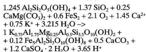
It must be noted that pyrite oxidation is not bound to this particular stage but also occurs earlier, whereby most of the Fe is forming ferric iron hydroxides responsible for the rusty discoloration. The sulphate derived from pyrite oxidation is highly soluble in the solution such that saturation with respect to gypsum is attained at later stages.
