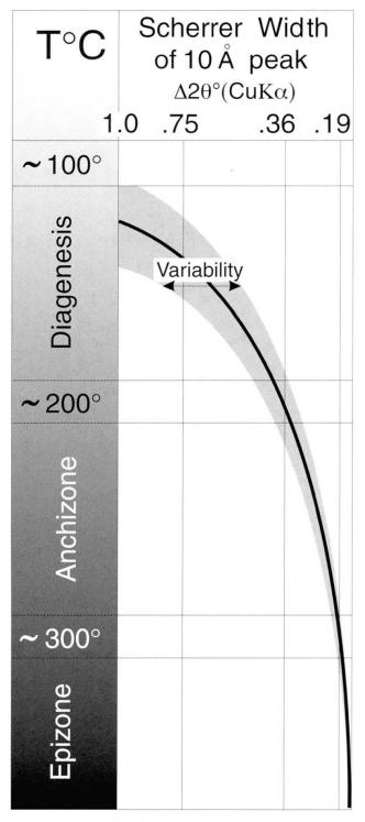
Fig. 4 FWHM (or Scherrer width)-temperature relation curve. The  $0.19^{\circ}$  and  $0.36^{\circ}$   $\Delta 2\theta^{\circ}$  (CuKα) are the upper and lower anchizonal boundary limits of the X-ray laboratory (Rigaku diffractometer) of the Inst. Mineral. and Petro., Univ. Lausanne. Modified after JABOYEDOFF and THÉLIN (1996) and references therein.
