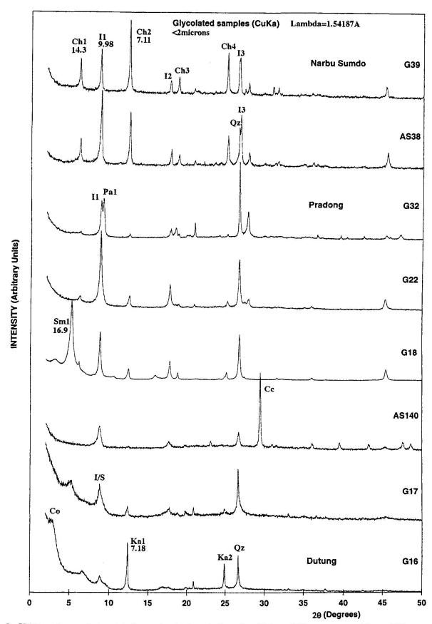
Fig. 3 XRD patterns of glycolated samples (< 2  $\mu$ m). Samples G16 to G39 are arranged from SW to NE (see Fig. 2 for a more precise location). Cc = calcite; Chl = chlorite; Co = corrensite; I = illite; I/S = illite/smectite mixed-layered clay mineral; Ka = kaolinite (presence confirmed by hydrazine test); Pa = paragonite; Sm = smectite. 1,2,3,4 indicate the order of the 00l reflection.
