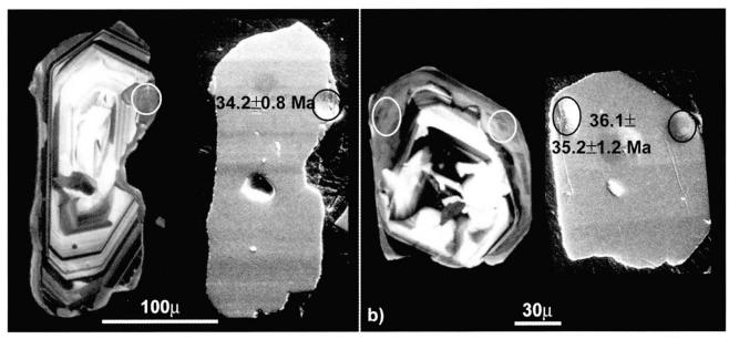
Fig. 3 Cathodoluminescence image (left) and secondary electron image (right) of two zircons dated. The Late Eocene/Early Oligocene rims are unzoned or irregularly zoned and have Th/U ratios below 0.01.
