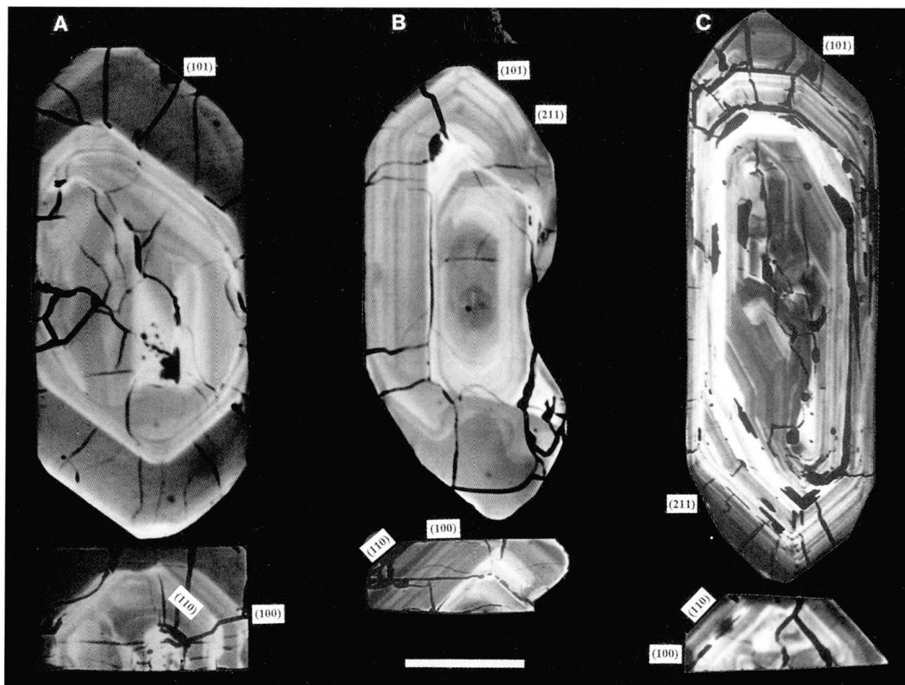
Fig. 4 Longitudinal and cross sections of zircons from the Schlieren-Granite. The prism evolution is characterized by a growth inhibition of the F-face  $\{100\}$  that leads to a clear predominance of this face in the outermost layer. Pyramidal development shows large  $\{101\}$  faces that only decrease slightly over the entire growth period. Bar = 30  $\mu\text{m}$ .
