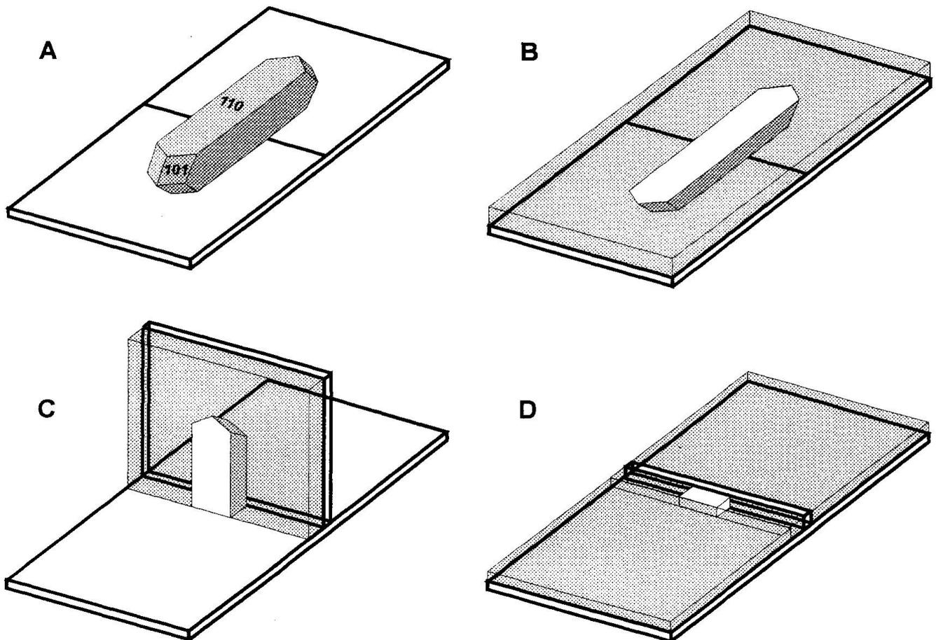
Fig. 1 Procedure of the preparation technique. (A) Crystals are oriented with their *c*-axes parallel to the longer side of the glass slide and fixed with resin. (B) Crystals are polished until their median sections are reached. (C) After microprobe work, longitudinal sections are halved and fixed on another slide. (D) Crystals are polished perpendicular to their *c*-axes. The final cross sections are 30 to 50 µm thick.
