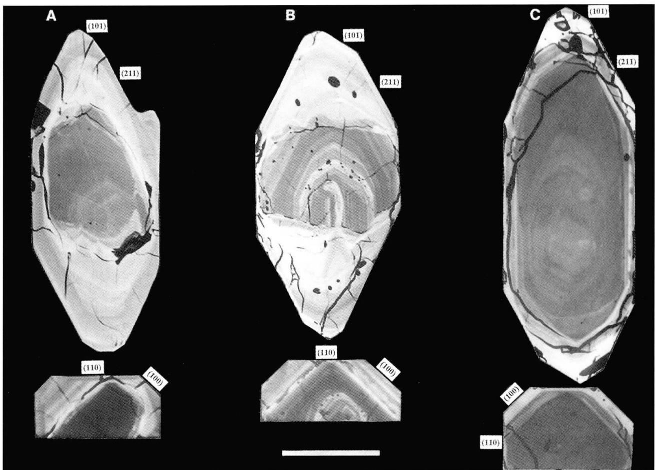
Fig. 3 Longitudinal and cross sections of zircons from the Pearl-Gneiss. While the evolution of the prism faces (below) is marked by a growth inhibition and final predominance of {110}, the pyramidal development starts with {101} faces that are in the same order of magnitude as {211} faces (A and B) and decrease continuously because of their higher growth speed. Bar = 30  $\mu$ m.
