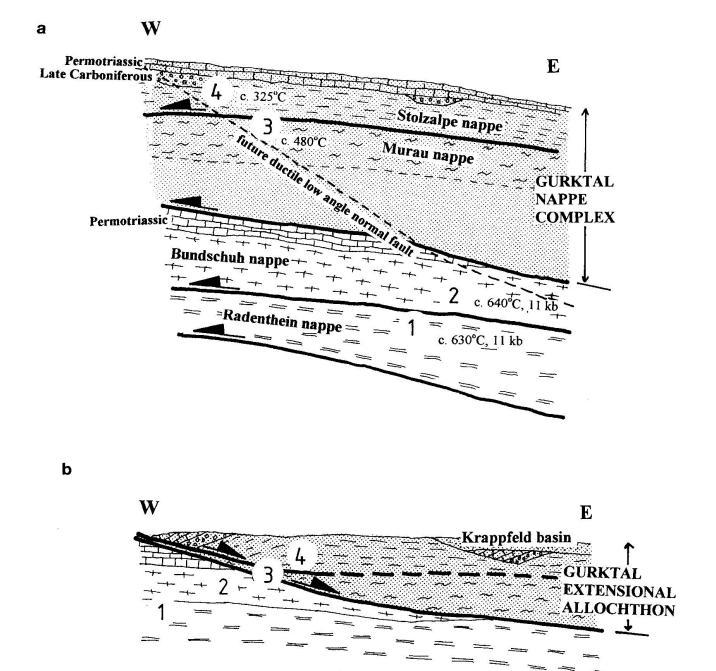
Fig. 10 Models of the tectonic evolution along the western margin of the Gurktal nappe complex. (a) Nappe stacking at the stage of maximum peak metamorphic conditions in the Bundschuh and Radenthein nappes. (b) Stage after extension by east-directed ductile low-angle normal faulting. 1–4 represent suggested locations at Cretaceous peak metamorphic conditions (a) and post-extensional locations (b) within all four investigated structural units.
