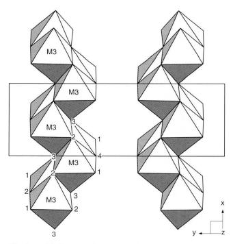
Fig. 2  $\alpha$ -PbO<sub>2</sub>-type zigzag double chains of edge-sharing M3O<sub>6</sub> octahedra extending in the [100] direction.
