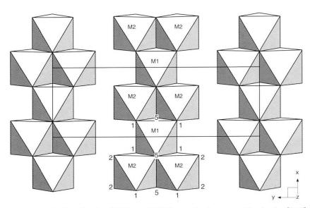
Fig. 1  $V_3O_5$ -type columns of edge-sharing M1O<sub>6</sub> and M2O<sub>6</sub> octahedra extending in the [100] direction which are alternatingly one and two octahedra wide.
