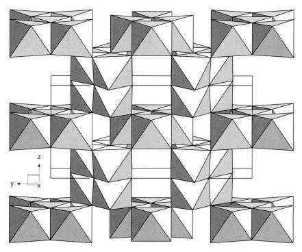
Fig. 3 The crystal structure of graeserite viewed approximately along [001]. The structure consists of layers of  $\alpha$ -PbO<sub>2</sub>-type double chains and V<sub>3</sub>O<sub>5</sub>-type columns, stacked in the [001] direction, as shown in the figures 1 and 2. Channels of cuboctahedral cavities extend through the structure along [100] containing (As,Sb) and Pb (cf. Fig. 4).
