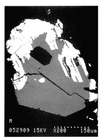
Fig. 3 BSE-image of quadratite (dark grey), jordanite (light grey), and pyrite (black idiomorphic inclusion). Diameter of sample about 0.3 mm.
