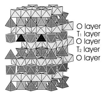
Fig. 1 Polyhedral representation of the zincohögbomite-8H structure. O-type octahedral layers are light gray with dark rims.  $T_2$ -type spinel layers are dark gray with black rims and nolanite-like  $T_1$  layers have light rims.
