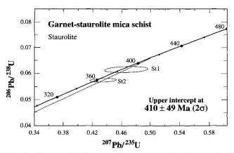
Fig. 4 Concordia diagram for staurolite bulk-samples St1 and St2. The contrasting  $^{206}\text{Pb}/^{238}\text{U}$  age of the two fractions indicates lead loss. The intercept age of  $410 \pm 49$  Ma is calculated from a discordia fitted through the origin of the diagram and represents a minimum age.
