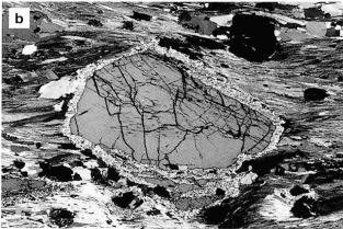
Fig. 2 Microphotograph of syntectonic staurolite with inclusion trails of ilmenite, rutile, and graphite aligned in the D2 foliation along with garnet, biotite, muscovite, plagioclase, and quartz. Photograph with crossed nicols distinctly shows decomposition of the staurolite to chlorite and mica at its rim. Length of lower edge is 7 mm.
