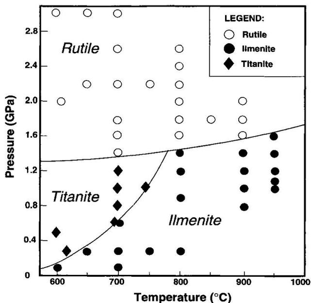
Fig. 2 Experimentally determined relations of rutile, titanite, and ilmenite for a tholeiitic basalt composition. These phases were identified in the run products and the P-T field boundaries were not reversed, hence should be considered as synthesis boundaries.
