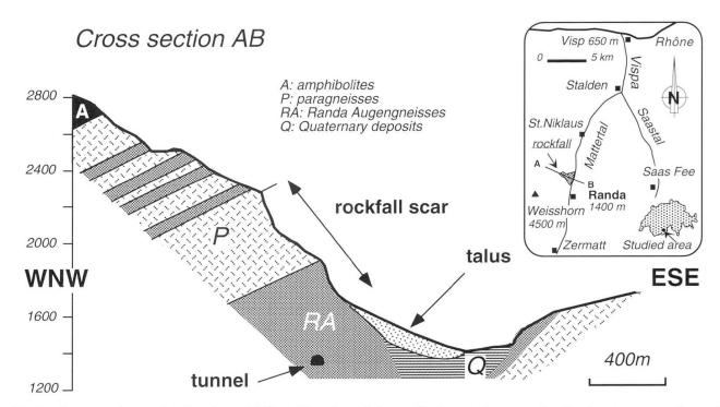
Fig. 3 Cross section at the Randa rockfall and location of the studied area. For more details about cross sections of the rockfall, see figure 3 from SCHINDLER et al. (1993).
