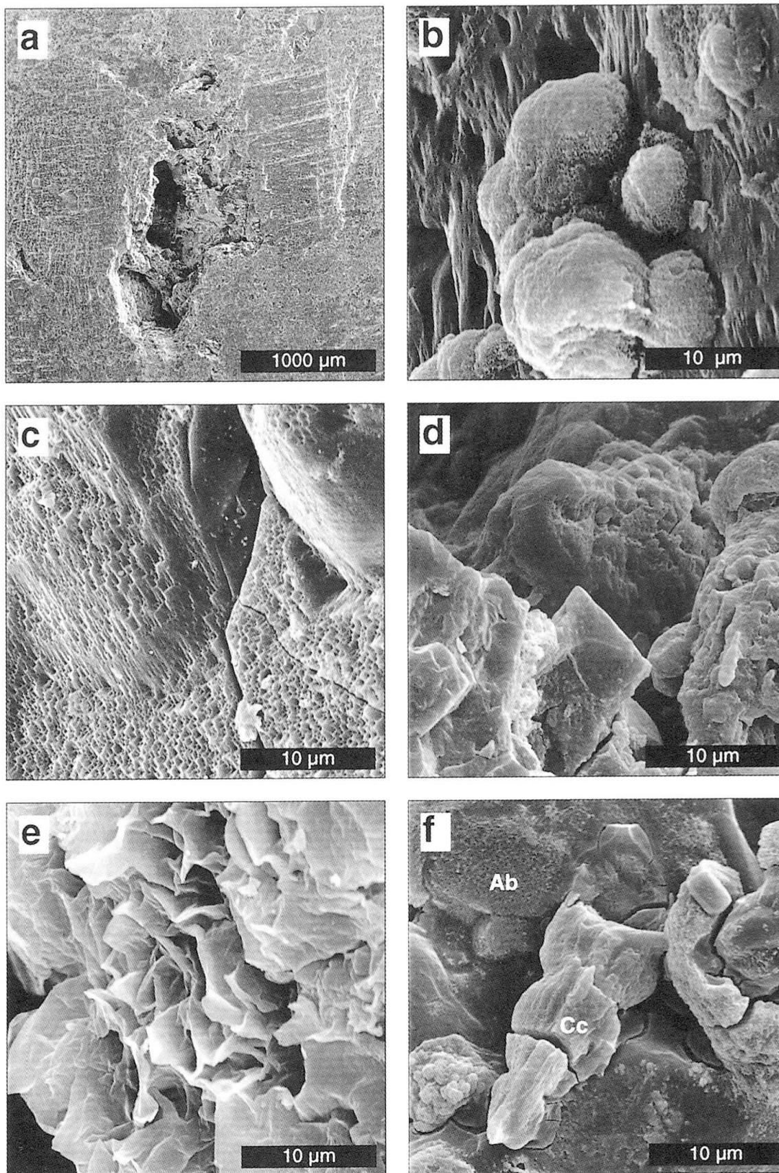
*Fig. 5* SEM images of the pores (SEI, 20 kV): (a) general view of a millimetric pore (FG24); (b) Fe and Mn rich pellets on a pitted quartz grain surface (FG24); (c) etch pits on quartz (FG24); (d) dissolution of K-feldspar (FG130); (e) smectite in K-feldspar (FG19); (f) residue of calcite grains on a feldspar surface (Cc: calcite; Ab: albite; FG130).
